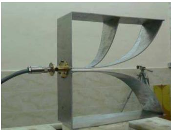
**Figure 5.** Fabricated antenna.
