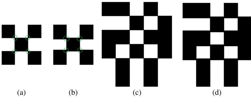
**Figure 5.** (a) Traditional on/off building blocks with infinitesimal connections. (b) Proposed overlapping scheme based on shifting of cells along the vertical axis. (c) A possible structure with infinitesimal connections. (d) A possible structure with overlapping as proposed in this paper.
