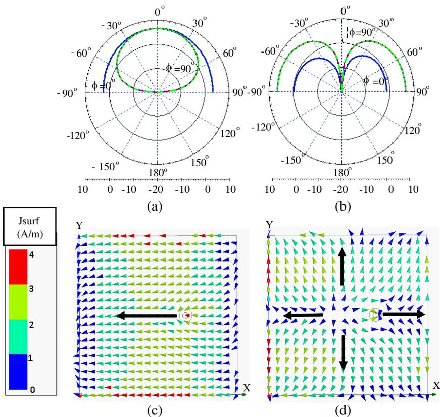
**Figure 2.** Simulation results of a square shaped patch. (a) Main radiation cuts at 1.98 GHz. (b) Main radiation cuts at 3.95 GHz. (c) Current distribution at 1.98 GHz. (d) Current distribution at 3.95 GHz. (The black arrow indicates the direction of current).
