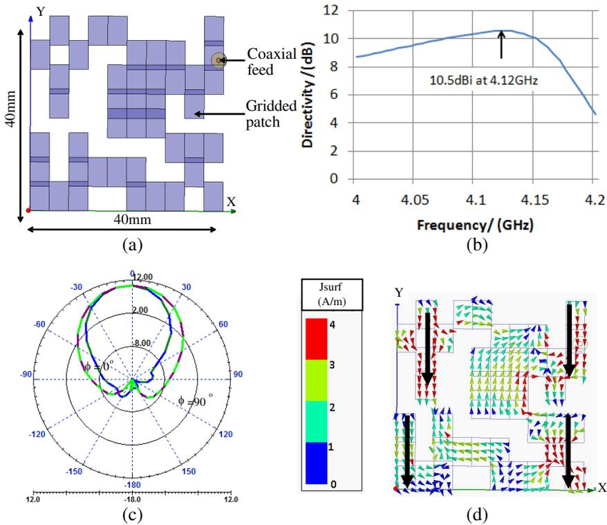
**Figure 7.** Simulation results of the optimized patch. (a) Patch geometry. (b) Directivity Vs Frequency. (c) Main radiation cuts at 4.12 GHz. (d) Current Distribution at 4.12 GHz showing the in-phase portions. (The black arrow indicates the direction of current).
