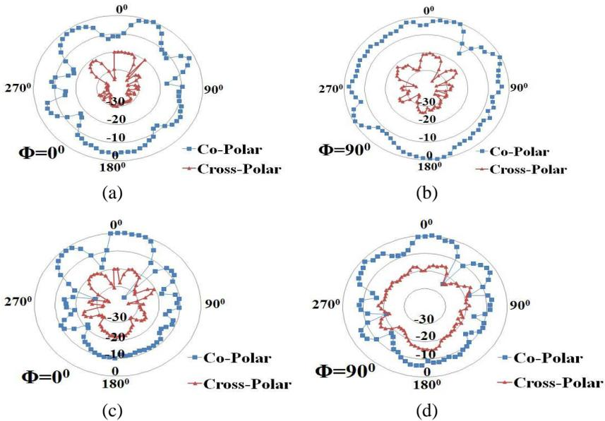
**Figure 11.** The radiation pattern as measured for the half HDRA with array of slots. The angles marked represent the ' $\theta$ ' plane. (a) (c)  $x$ - $z$  plane ( $\Phi = 0^\circ$ ). (b) (d)  $y$ - $z$  plane ( $\Phi = 90^\circ$ ). (a) (b) 5.74 GHz. (c) (d) 6.02 GHz.
