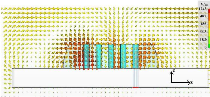
**Figure 5.** The Electric Field distribution of the half HDRA with periodic holes at 6.08 GHz. The Blue coloured cylinders are the holes drilled in the half HDRA. The arrows show the orientation of the electric field.
