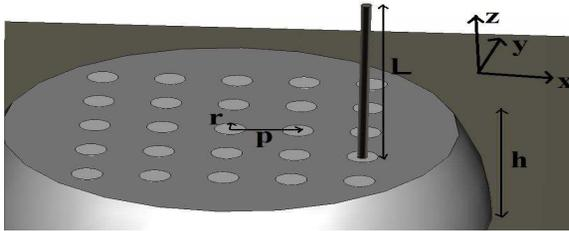
**Figure 1.** The proposed structure with radius ‘ $r$ ’ and periodicity ‘ $p$ ’ of the drilled holes. The probe is increased by length ‘ $L$ ’ and ‘ $h$ ’ is the height of the HDRA. For the above case, ‘ $L$ ’ is zero.
