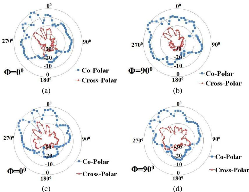
**Figure 14.** The radiation pattern as measured for the half HDRA with extended probe length of  $L = 2.5$  cm. The angles marked represent the ‘ $\theta$ ’ plane. (a) (c)  $x$ - $z$  plane ( $\Phi=0^\circ$ ). (b) (d)  $y$ - $z$  plane ( $\Phi = 90^\circ$ ). (a) (b) 4.5 GHz. (c) (d) 5 GHz.
