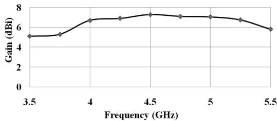
**Figure 15.** The gain vs. Frequency plot for the half HDRA with periodic slots and extended probe length of  $L = 2.5$  cm.
