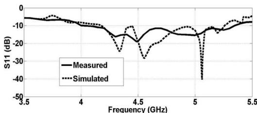
**Figure 13.** Plot of the measured and simulated return loss for the half HDRA with extended probe length of  $L = 2.5$  cm. The 10 dB bandwidth measured is 1.3 GHz.
