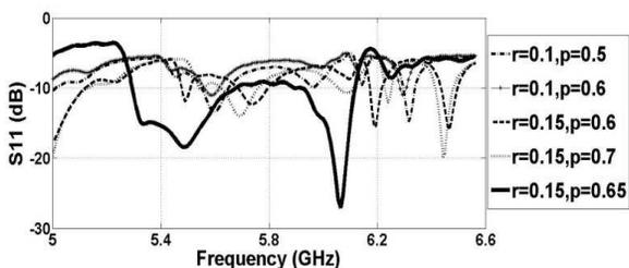
**Figure 3.** The parametric analysis to optimize the value of the drilled holes of radius ‘ $r$ ’ and the periodicity ‘ $p$ ’ of the repetition of the holes. All measurements of ‘ $r$ ’ and ‘ $p$ ’ are in cms.
