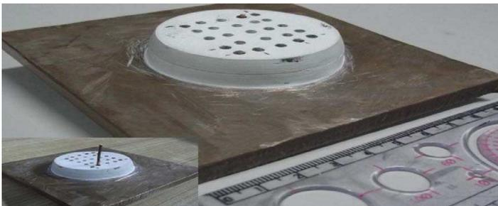
**Figure 8.** The side view of the fabricated structure of half HDRA with probe feed. The inset picture shows the side view of the fabricated structure of half HDRA with extended probe feed of length  $L = 2.5$  cms.
