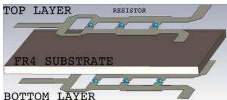
**Figure 4.** Wideband WPD architecture (the metal strips have been detached from the substrate in order to enhance the visibility of the structure, the lumped resistors are drawn in blue).
