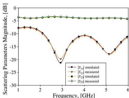
**Figure 13.** Comparison of simulated and measured  $|S_{11}|$ ,  $|S_{21}|$  for proposed WPD.
