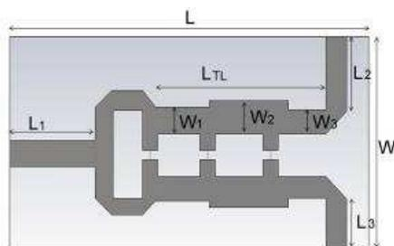
**Figure 5.** Wideband WPD parameters notation (top view).
