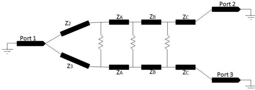
**Figure 2.** Transmission line model of the modified/proposed WPD.
