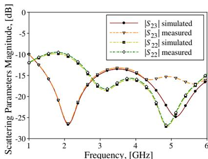
**Figure 14.** Comparison of simulated and measured  $|S_{22}|$ ,  $|S_{23}|$  for the proposed WPD.
