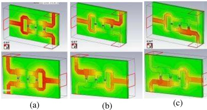
**Figure 11.** Current distribution at 2.45 GHz: (a) Current distribute equally to port 2 & 3; (b) Isolate port 3; (c) Isolate port 2.
