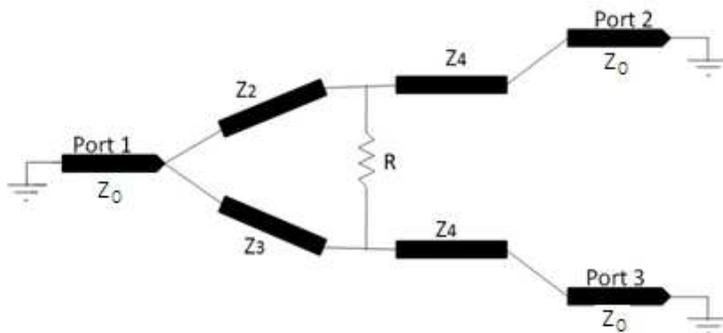
**Figure 1.** Transmission line model of the normal WPD.
