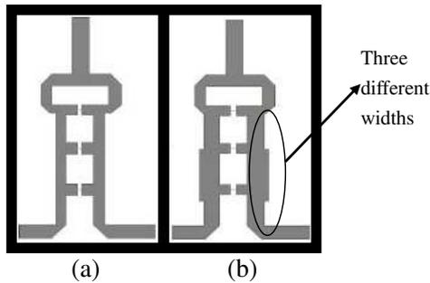
**Figure 3.** (a) Initial design of proposed WPD; (b) Final design of proposed WPD.
