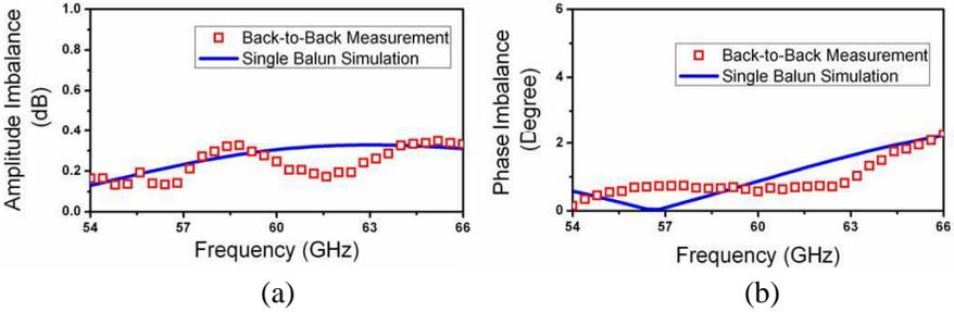
**Figure 5.** The extracted amplitude and phase imbalances from the two back-to-back measurements and compared with single balun simulated results. (a) Amplitude imbalance. (b) Phase imbalance.
