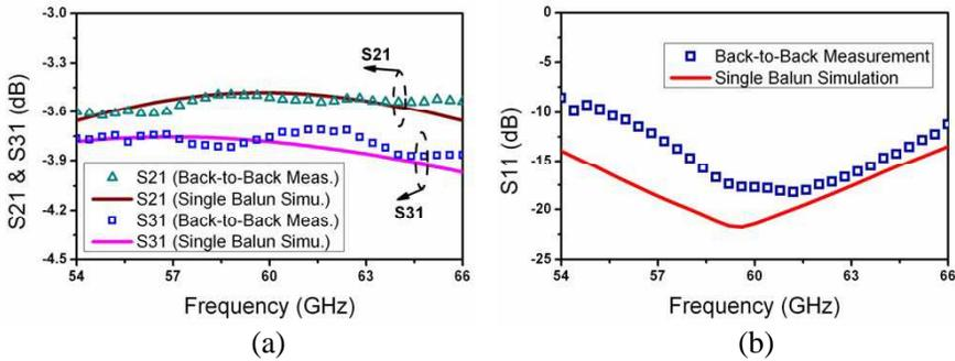
**Figure 4.** The extracted  $S$ -parameter results from the two back-to-back measurements and compared with single balun simulated results. (a)  $S_{21}$  and  $S_{31}$ . (b)  $S_{11}$ .
