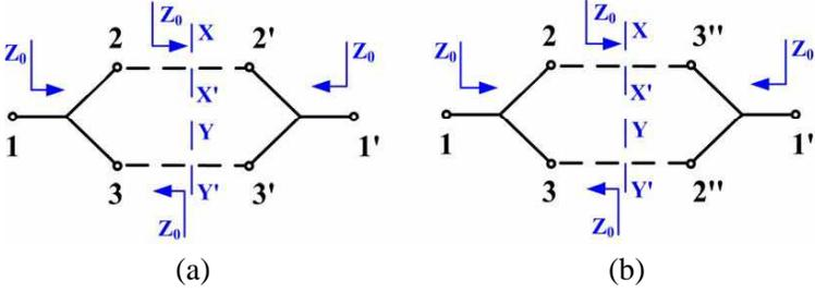
**Figure 2.** Block diagram of the two different back-to-back connection ways of two identical baluns. (a) The one with port 2 to port 2, port 3 to port 3. (b) The one with port 2 to port 3, port 3 to port 2.
