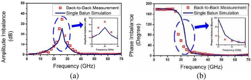
**Figure 6.** The extracted amplitude and phase imbalances from the two back-to-back measurements and compared with single balun simulated results from 2 GHz to 70 GHz. (a) Amplitude imbalance. (b) Phase imbalance.
