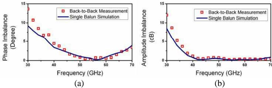
**Figure 7.** The extracted amplitude and phase imbalances from the two back-to-back measurements and compared with single balun simulated results from 30 GHz to 70 GHz. (a) Amplitude imbalance. (b) Phase imbalance.
