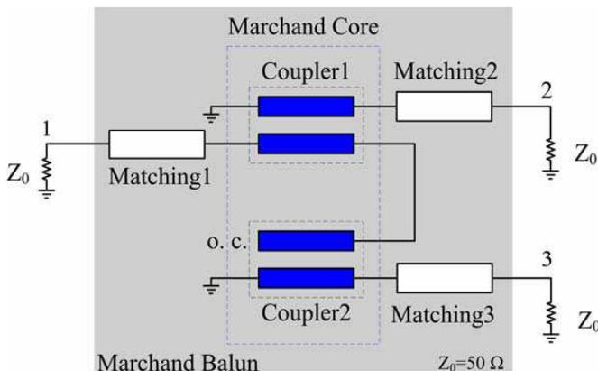
**Figure 1.** Block diagram of a Marchand balun as two identical couplers with port impedance matching.
