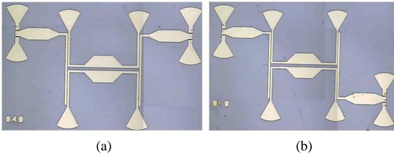
**Figure 3.** Microphotographs of the two different back-to-back connection ways of two identical baluns. (a) The one with port 2 to port 2, port 3 to port 3. (b) The one with port 2 to port 3, port 3 to port 2.
