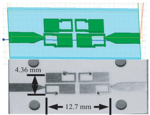
**Figure 7.** Simulation model of the multilayered filter.
