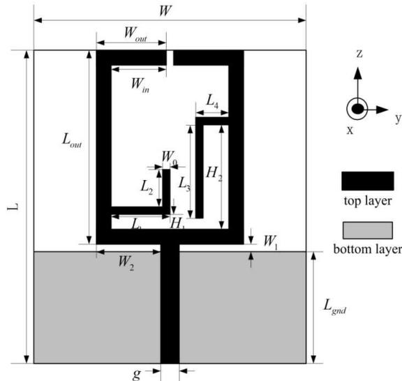
**Figure 1.** Configuration of the proposed antenna.
