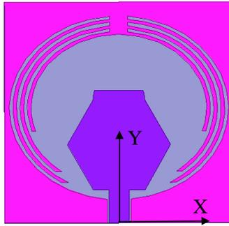
**Figure 5.** The structure of multiband antenna.
