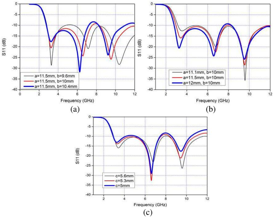
**Figure 2.** Simulated reflection coefficients of the primitive antenna for (a) variance of  $b$  ( $a = 11.5$  mm and  $c = 5.66$  mm), (b) variance of  $a$  ( $b = 10$  mm and  $c = 5.6$  mm), (c) variance of  $c$  ( $a = 11.5$  mm and  $b = 10$  mm).
