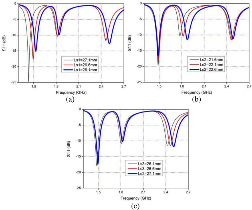
**Figure 4.** The simulated reflection coefficients of the multi-band antenna with (a)  $L_{s2} = 22.1$  mm and  $L_{s3} = 16.1$  mm for various  $L_{s1}$ , (b)  $L_{s1} = 26.6$  mm and  $L_{s3} = 16.1$  mm for various  $L_{s2}$ , (c)  $L_{s1} = 26.6$  mm and  $L_{s2} = 22.1$  mm for various  $L_{s3}$ .
