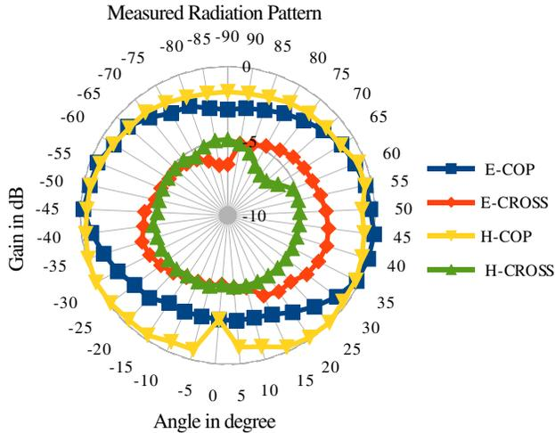
**Figure 10.** Measured radiation patterns at 10.8 GHz.
