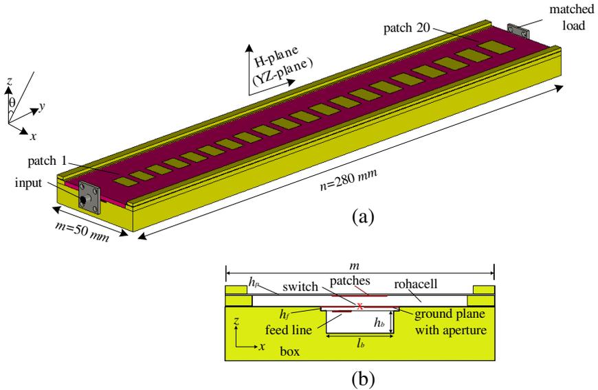
**Figure 5.** Proposed antenna structure. (a) Perspective view. (b) Side view.  $\tau = 1.02$ ,  $\epsilon_r = 2.2$  (for  $h_f$  and  $h_p$ ),  $\epsilon_r = 1.09$  (for rohacell),  $w_f = 2.38$  mm,  $h_f = 0.787$  mm,  $h_p = 0.254$  mm, rohacell = 2 mm,  $d_1 = 16.1$  mm,  $\sigma = 15.86$  mm,  $w_1 = 7$  mm,  $l_1 = 10.77$  mm.
