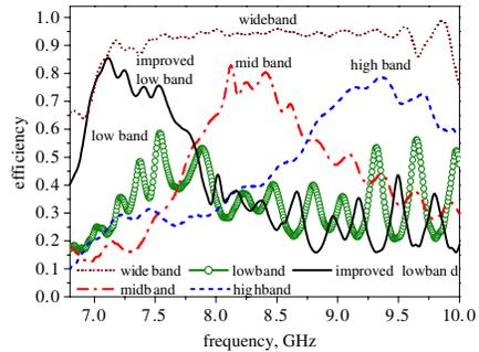
**Figure 8.** Simulated efficiency for selected four frequency bands.
