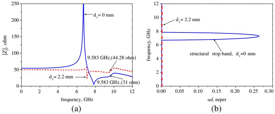
**Figure 4.** (a) Image impedance,  $|Z_i|$ . (b) Attenuation,  $ad$ .
