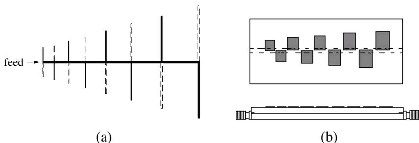
**Figure 1.** (a) Log periodic printed dipole array [8]. (b) An electromagnetic coupled patch array [15].
