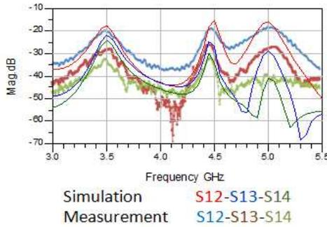
**Figure 9.** The  $1 \times 4$  array coupling coefficients  $S_{12}$ ,  $S_{13}$ ,  $S_{14}$ .
