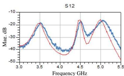
Figure 6. The  $1 \times 2$  array coupling coefficients.
