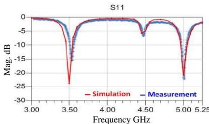
**Figure 2.** Single element reflection coefficient  $S_{11}$ .
