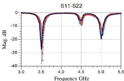
Figure 5. The  $1 \times 2$  array reflection coefficients.
