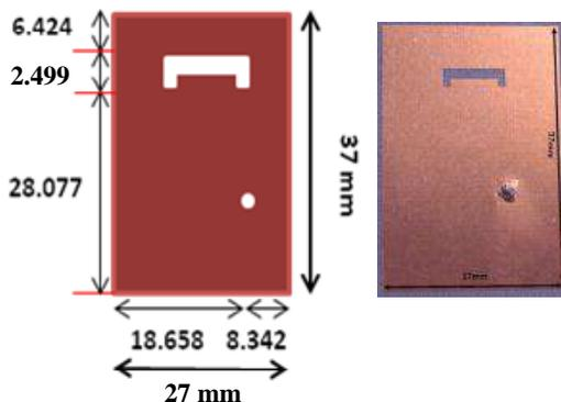
**Figure 1.** Geometry of a U-slotted antenna element.
