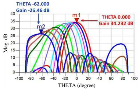
**Figure 11.** The  $4 \times 4$  planar array beam steering.
