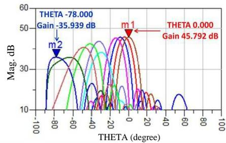
**Figure 13.** The  $8 \times 8$  planar array beam steering.
