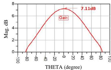
**Figure 3.** Single element gain.
