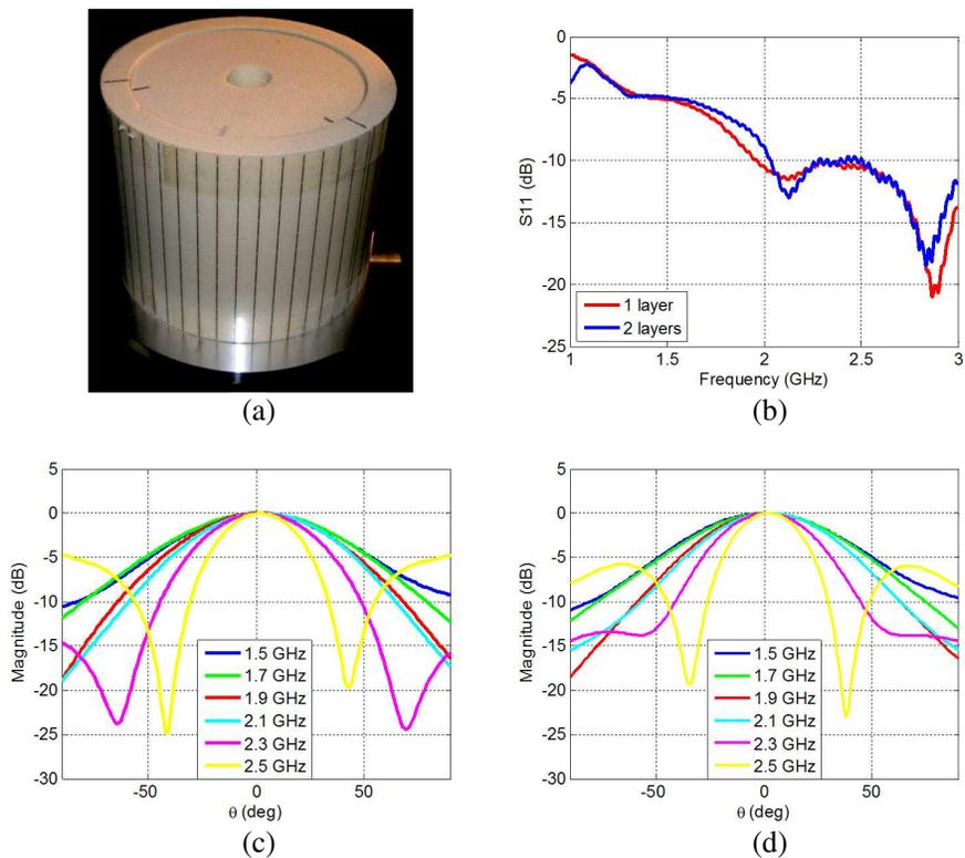
**Figure 6.** (a) Photograph of the fabricated antenna. (b) Measured  $S_{11}$  parameter of the base station antenna with a metamaterial composed of one and two layers. (c)–(d) Measured  $H$ -plane radiation patterns for metamaterial with respectively one layer and two layers.
