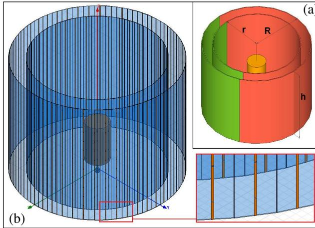
**Figure 3.** (a) Schematic view of the two metasurface-layer antenna with the discontinuous wires zone (green) and the continuous one (red). (b) Design incorporating continuous and discontinuous wires used in the simulation process. The inset shows the discontinuous wires in the design.
