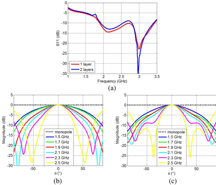
**Figure 5.** (a) Simulated  $S_{11}$  parameter of the base station antenna with a metamaterial made of one and two layers. (b)–(c) Simulated  $H$ -plane radiation patterns for respectively one layer and two metamaterial layers.
