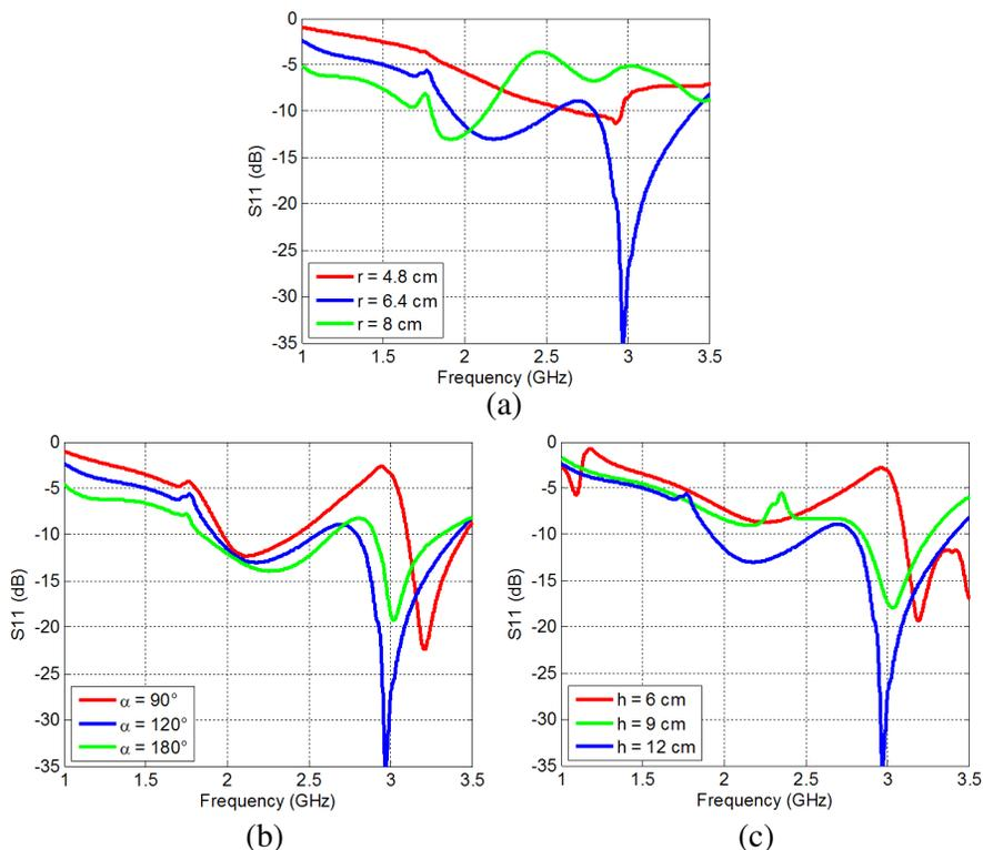
**Figure 4.** Optimization of the design parameters  $r$ ,  $\alpha$  and  $h$  for best tradeoff in impedance matching with  $R - r = 1.6\text{ cm}$ . (a)  $r$  varying with  $\alpha = 120^\circ$  and  $h = 12\text{ cm}$ . (b)  $\alpha$  varying with  $r = 6.4\text{ cm}$  and  $h = 12\text{ cm}$ . (c)  $h$  varying with  $\alpha = 120^\circ$  and  $r = 6.4\text{ cm}$ .
