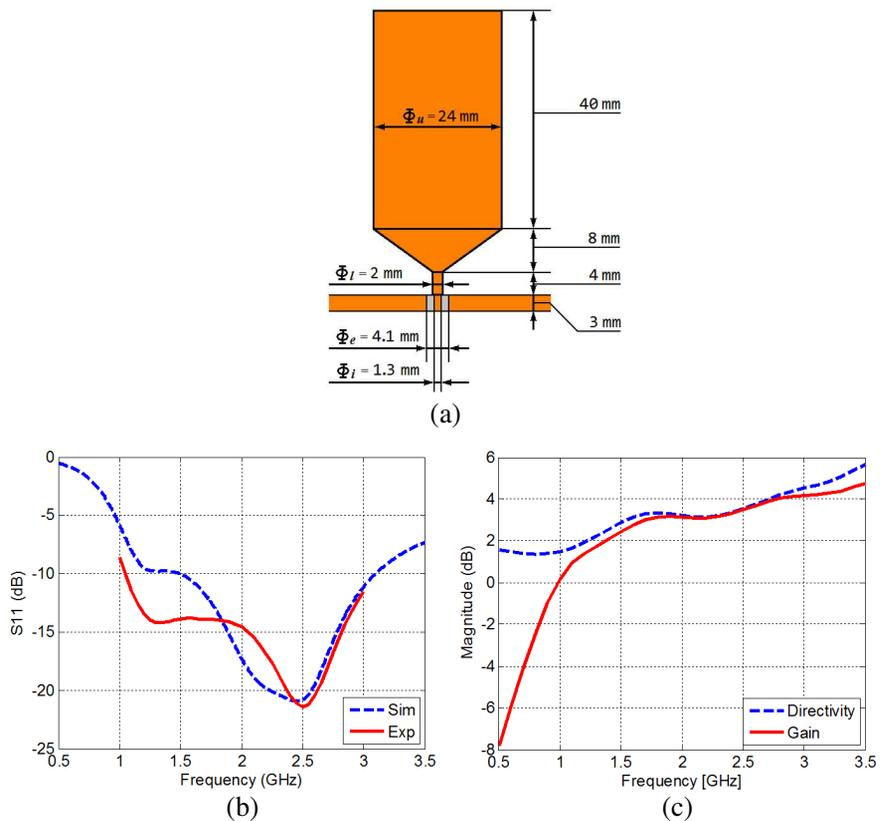
**Figure 1.** (a) Schematic view of the conical monopole primary source. (b) Simulated and measured  $S_{11}$  parameter. (c) Simulated directivity and gain.
