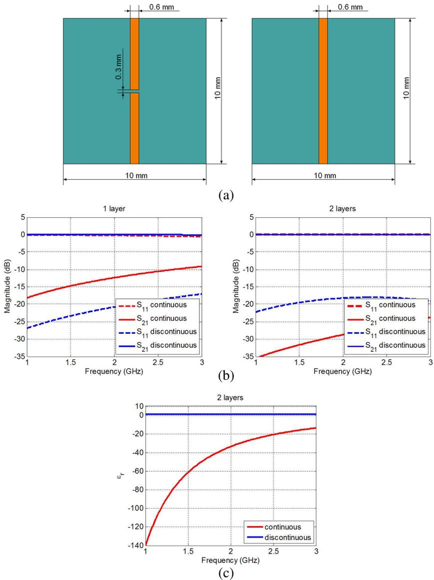
**Figure 2.** (a) Elementary cells of a lattice made of a layer of respectively continuous and discontinuous metallic strips. (b)  $S$ -parameters of one and two layers of both lattices for a normal incident wave with the  $E$ -field parallel to the strips. (c) Effective permittivities of the two layers with continuous (red curve) and discontinuous wires (blue curve).
