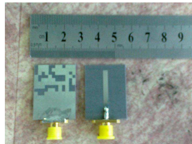
Figure 5. Best antenna made using the result of optimization.
