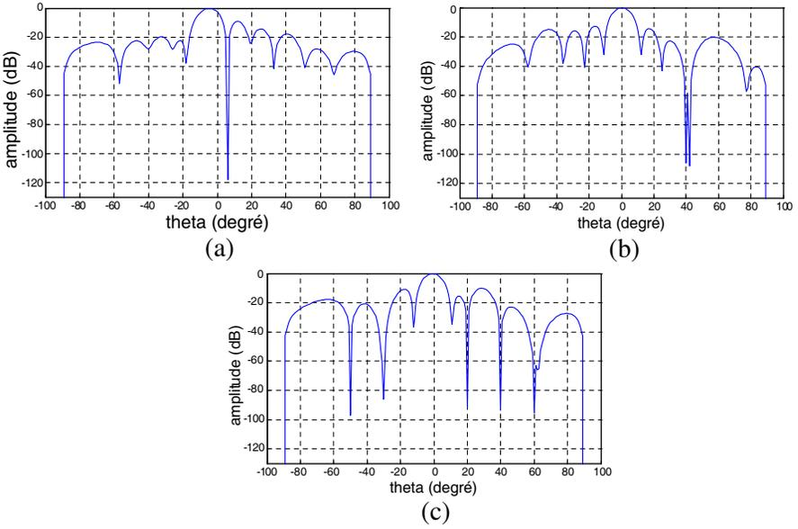
**Figure 2.** Interferences rejections by HBMO/TS: (a) interference rejection in the direction of the main lobe at  $6^\circ$ , (b) two very closed interferences rejections at  $40^\circ$  and  $42^\circ$ , (c) the case of several interferences rejections (interferences at  $-50^\circ$ ,  $-30^\circ$ ,  $20^\circ$ ,  $40^\circ$ ,  $60^\circ$ ).
