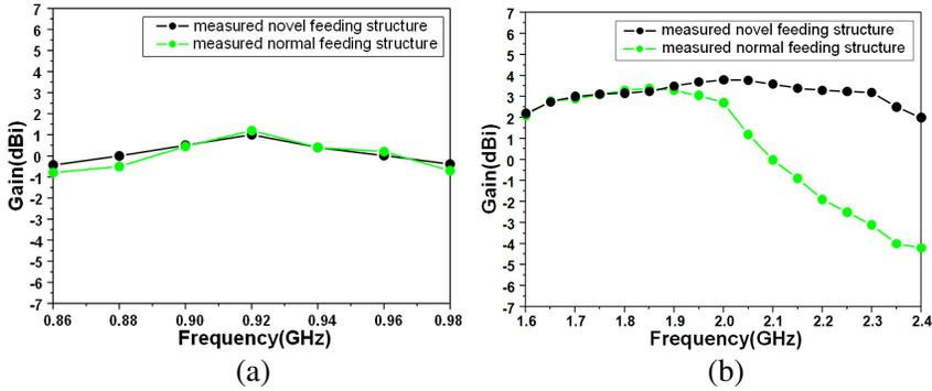
**Figure 6.** Measured gain and efficiency of the proposed antenna. (a) At low band, (b) at high band.
