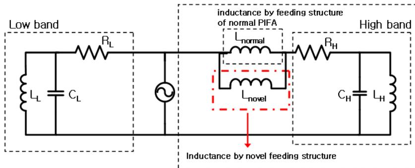
**Figure 4.** Equivalent circuit of novel feeding structure antenna.
