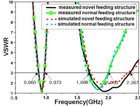
**Figure 2.** Simulation and measurement results on the VSWR of the proposed antenna.
