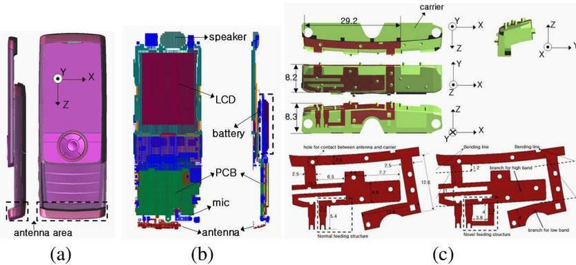
**Figure 1.** Geometry of practical handset and proposed antenna. (a) Handset feature, (b) metal part of the handset, (c) feature of the proposed antenna.
