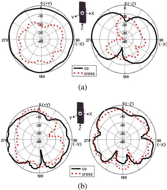
**Figure 5.** Measured radiation patterns of the proposed antenna. (a) 0.9 GHz at low band, (b) 2,000 MHz at high band.
