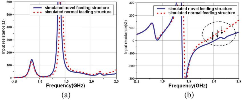
**Figure 3.** Simulation results on the input impedance of the proposed antenna. (a) Resistance, (b) reactance.
