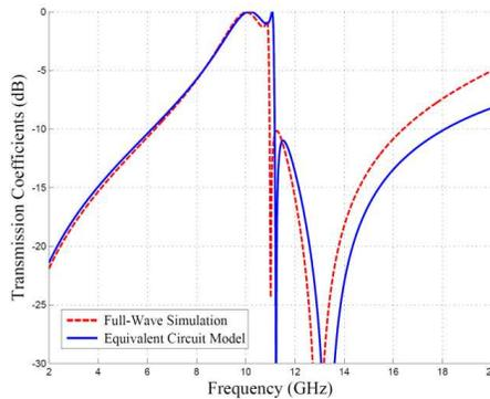
**Figure 6.** Transmission coefficient of the second-order bandpass MEFSS. Full-wave simulation by CST and equivalent circuit analyzed by ADS (Figure 5), where the element values are according to the Table 3.
