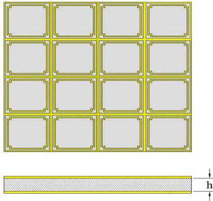
**Figure 1.** Top and side views of the bandpass MEFSS etched on the two side of a Taconic RF-35 dielectric substrate with the characteristics of  $\epsilon_r = 3.5$ ,  $\tan \delta = 0.0018$  and thickness of  $h = 0.762$  mm.
