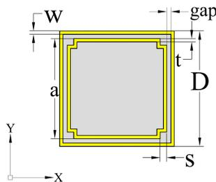
**Figure 2.** The unit cell of the FSS shown in Figure 1. Each unit cell is composed of a single LC loop inside a section of the mesh grid. The structure is designed to be polarization insensitive at normal incidence.
