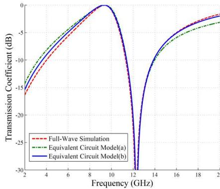
**Figure 4.** Transmission Coefficients of the MEFSS depicted in Figure 2. ADS is employed for the simulation of equivalent circuit model shown on Figure 3, where the element values are according to the Table 2.
