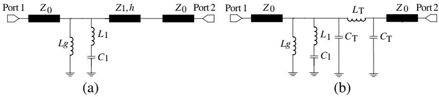
**Figure 3.** The equivalent circuit model for (a) the first-order bandpass MEFSS and (b) first-order bandpass MEFSS and dielectric substrate for normal incident waves.  $L_g$  is the wire grid inductances,  $C_T$  and  $L_T$  model the dielectric substrate [19].
