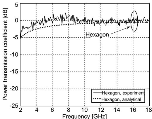
**Figure 6.** Comparison, in the 2–18 GHz band, between experimental data and the analytical approach, for the mesh with large hexagonal apertures. As discussed in the text, the numerical simulations are not performed for this case.
