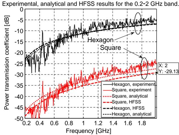
**Figure 5.** Comparison, in the 0.2–2 GHz band, between experimental data, analytical approach, and numerical simulations done with HFSS. The two cases are shown, mesh with small square apertures and mesh with large hexagonal apertures. As discussed in the text, the sharp peak around 400 MHz is deemed to be from leakage around the frame.
