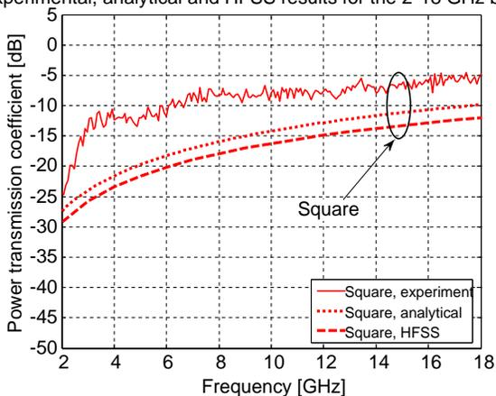
**Figure 7.** Comparison, in the 2–18 GHz band, between experimental data, analytical approach, and numerical simulations done with HFSS for mesh with square apertures. The difference between the experimental data and the two other datasets (for this case) is believed to be due to the  $Q$  value being too low, in the reference case, for useful comparison.
