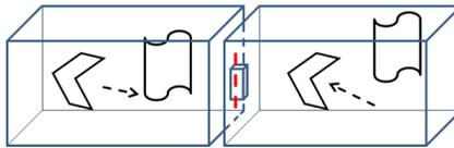
**Figure 4.** The cascaded reverberation chambers with the bridge, where the mesh is installed, shown.
