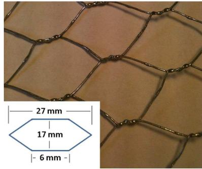
**Figure 1.** The mesh with hexagonal apertures.
