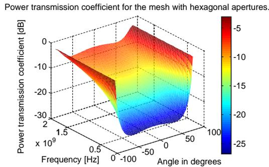
**Figure 3.** Using the method of an equivalent square area and (1b) the power transmission coefficient, as a function of frequency and angle of incidence, can be calculated for the mesh with hexagonal apertures.
