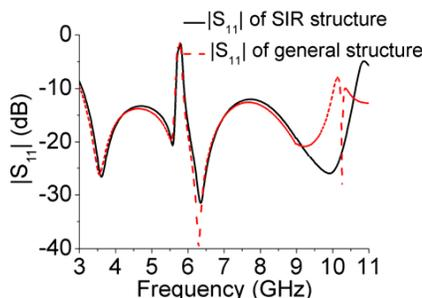
**Figure 18.** Simulated  $|S_{11}|$  with UR and SIR structure.
