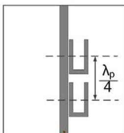
**Figure 10.** Traditional structure of two order band-stop filter.
