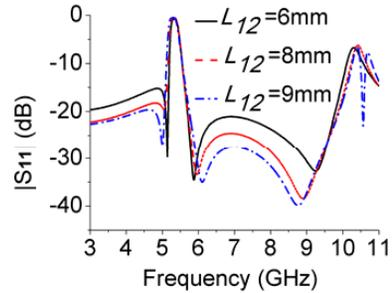
Figure 16.  $|S_{11}|$  for different  $L_{12}$ .
