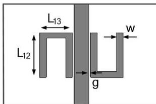
**Figure 11.** Geometry of the proposed band-stop filter.
