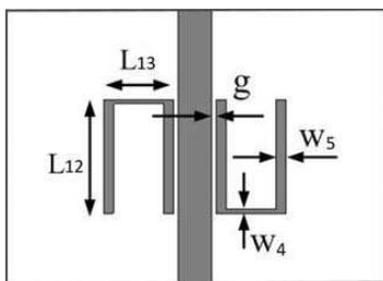
**Figure 17.** Two order band-stop filter with SIR structure.
