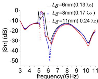
**Figure 6.** Simulated  $|S_{11}|$  with different  $L_6$ .
