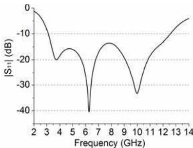
**Figure 3.** Return loss of the UWB antenna without band-rejected structure.
