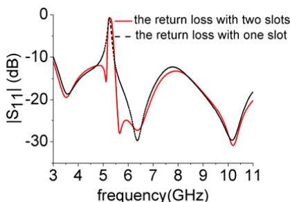
**Figure 5.** Simulated  $|S_{11}|$  with one and two slits.
