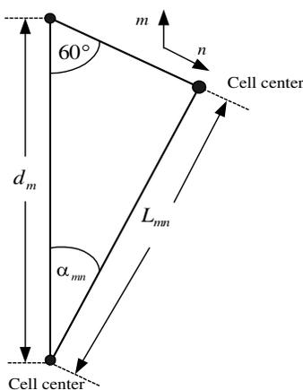
Figure 8. Coordinate system for cell location determination.
