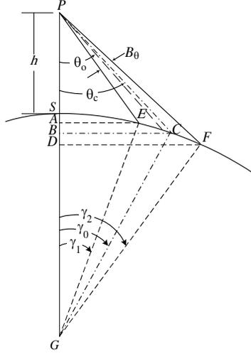
**Figure 3.** Curved earth coverage geometry.
