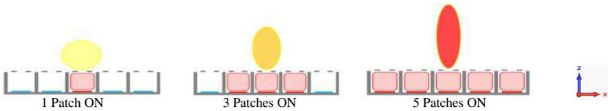
**Figure 11.** Principle of the directivity/beam reconfigurable M-EBG antenna.
