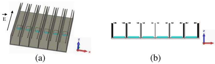
**Figure 4.** (a) Perspective and (b) inside views of the beam scanning M-EBG antenna.
