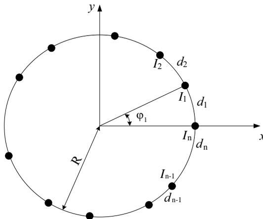
Figure 1. Geometry of  $N$ -element circular ring array.
