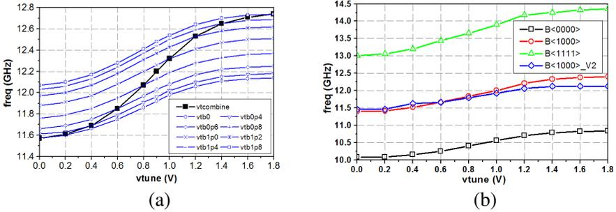
**Figure 6.** Tuning range. (a) Tuning curves of VCO1 with digital bits setting to  $\langle 1,0,0,1 \rangle$ . (b) Total tuning range of VCO1 (with control signals  $vtune$  and  $vtb$  combined), and tuning range of VCO2 with digital bits setting to  $\langle 1,0,0,0 \rangle$ .
