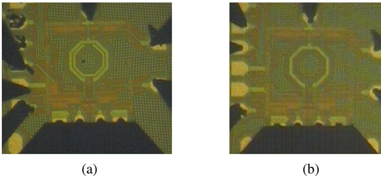
**Figure 3.** Die photos: (a) VCO1 with proposed magnetic coupled  $LC$  tanks; (b) VCO2 with normal  $LC$  tank and same parameter settings.
