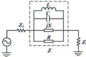
**Figure 10.** Equivalent circuit for the DP-EBG microstrip structure.
