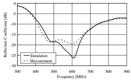
**Figure 8.** Reflection coefficient of the B-PSA. ( $L_{s1} = 48$ ,  $L_{s2} = 48$ ,  $L_{s3} = 96$ ,  $W_{s1} = 7$ ,  $W_{s2} = 40$ ,  $W_{s3} = 87$ ,  $L_g = W_g = 230$ ,  $L_d = 200$ ,  $h = 3$  mm,  $\epsilon_r = 7.35$ ).
