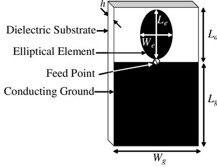
**Figure 2.** Structure of the B-PMA.
