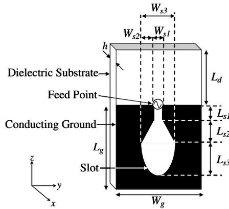
**Figure 6.** Structure of the B-PSA.
