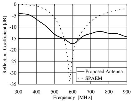
**Figure 10.** Simulated reflection coefficient. Proposed Antenna:  $L_e = 140$ ,  $W_e = 112$ ,  $e = 0.6$ ,  $L_{s1} = 48$ ,  $L_{s2} = 48$ ,  $L_{s3} = 96$ ,  $W_{s1} = 7$ ,  $W_{s2} = 40$ ,  $W_{s3} = 87$ ,  $L_g = W_g = 230$ ,  $L_d = 200$ ,  $h = 3$  mm,  $\epsilon_r = 7.35$ ).
