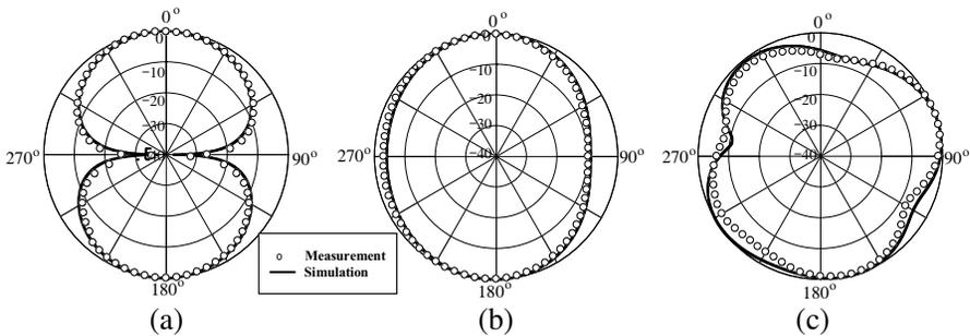
**Figure 12.** Co-polarized radiation patterns of the proposed antenna at 590 MHz. (a)  $E_\varphi$  in the  $xy$ -plane. (b)  $E_\varphi$  in the  $xz$ -plane. (c)  $E_\theta$  in the  $zy$ -plane.
