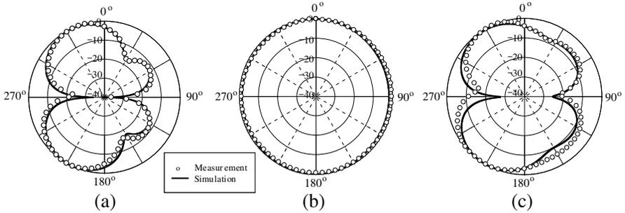
**Figure 5.** Co-polarized radiation patterns of the B-PMA at 590 MHz. (a)  $E_\varphi$  in the  $xy$ -plane. (b)  $E_\varphi$  in the  $xz$ -plane. (c)  $E_\theta$  in the  $zy$ -plane.
