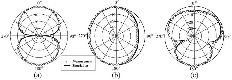
**Figure 9.** Co-polarized radiation patterns of the B-PSA at 590 MHz. (a)  $E_\varphi$  in the  $xy$ -plane. (b)  $E_\varphi$  in the  $xz$ -plane. (c)  $E_\theta$  in the  $zy$ -plane.
