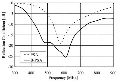
**Figure 7.** Simulated reflection coefficient. (B-PSA:  $L_{s1} = 48$ ,  $L_{s2} = 48$ ,  $L_{s3} = 96$ ,  $W_{s1} = 7$ ,  $W_{s2} = 40$ ,  $W_{s3} = 87$ ,  $L_g = W_g = 230$ ,  $L_d = 200$ ,  $h = 3$  mm,  $\epsilon_r = 7.35$ ).
