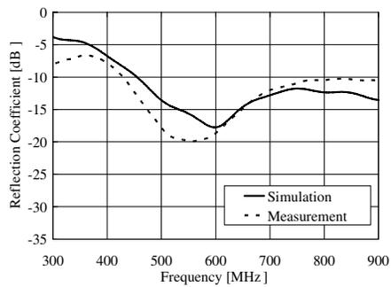
**Figure 11.** Reflection coefficient of the proposed antenna. ( $L_e = 140$ ,  $W_e = 112$ ,  $e = 0.6$ ,  $L_{s1} = 48$ ,  $L_{s2} = 48$ ,  $L_{s3} = 96$ ,  $W_{s1} = 7$ ,  $W_{s2} = 40$ ,  $W_{s3} = 87$ ,  $L_g = W_g = 230$ ,  $L_d = 200$ ,  $h = 3$  mm,  $\epsilon_r = 7.35$ ).
