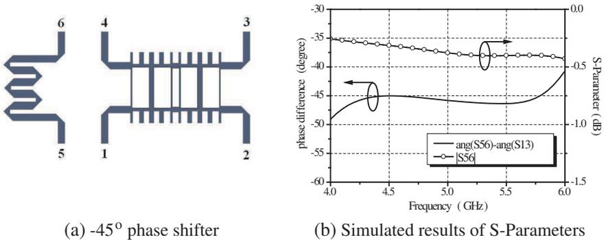
**Figure 7.**  $-45^\circ$  phase shifter and the simulated results.
