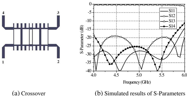
**Figure 6.** The crossover and the simulated results.
