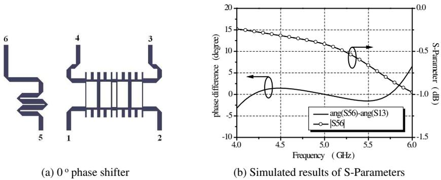
Figure 8.  $0^\circ$  phase shifter and the simulated results.
