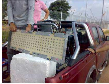
**Figure 10.** Measurement setup with microstrip array antenna.
