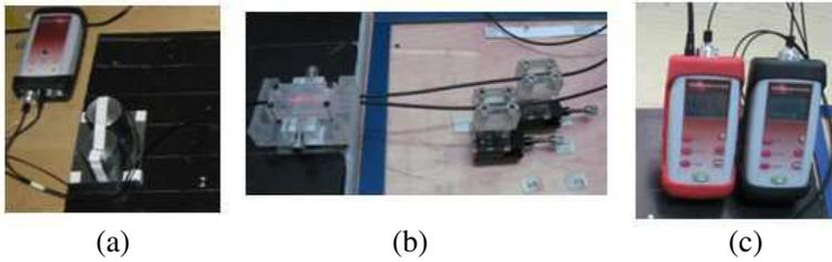
**Figure 14.** Setup for POF system coupling (a) optical source and mode scrambler, (b) device under-test and two miniature translation stages, (c) power meters.
