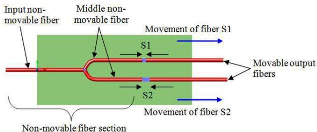
**Figure 4.** Generic Y-branch coupler with movable output fibers.
