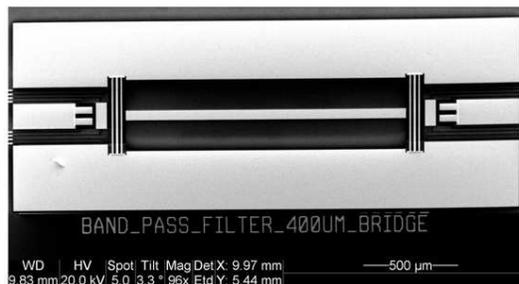
**Figure 9.** A SEM image of the fabricated band-pass filter.
