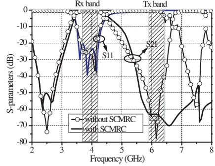
**Figure 6.** Simulated results of Rx-filter without SCMRC and with SCMRC.
