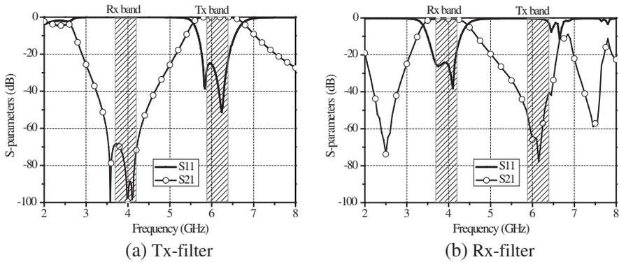
**Figure 2.** Simulation performance of the DBR filters.
