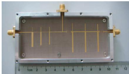
Figure 9. The photograph of the fabricated diplexer.
