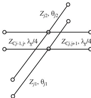
**Figure 1.** DBR filter based upon different-length open-circuited stubs.
