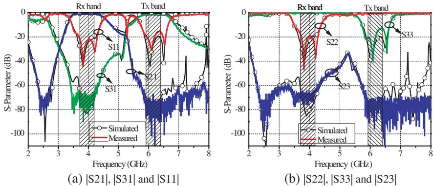
**Figure 10.** Simulated and measured  $S$ -parameters of the proposed diplexer.
