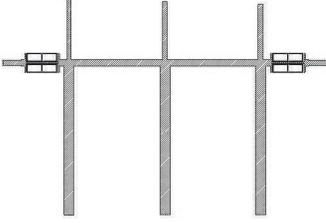
**Figure 5.** Layout of Rx-filter with SCMRC.
