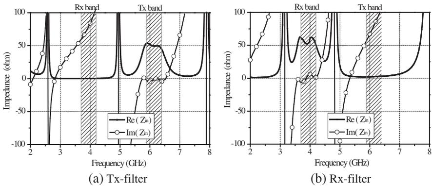
Figure 7. Input impedances of Tx and Rx filters.
