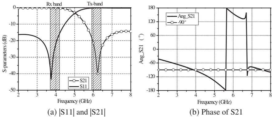
Figure 4. Simulated  $S$ -parameters of SCMRC.
