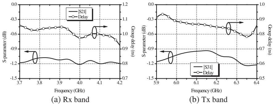
**Figure 11.** Measured insertion loss and group delay of the proposed diplexer in Rx/Tx band.
