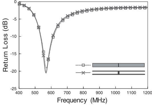
**Figure 2.** Comparison of the simulated return loss between the two-rectangular patches dipole antenna and the back-to-back symmetric dual-C-shape uniform strips dipole antenna.
