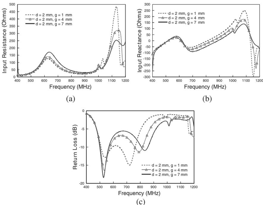
**Figure 4.** Simulated the variation of  $g$  of the gap between back to back asymmetric dual-C-shape strips ( $d = 2$  mm). (a) Resistance of the proposed antenna for variation in  $g$ . (b) Reactance of the proposed antenna for variation in  $g$ . (c) Simulated return loss as a function of distance  $g$ . Other dimensions are the same as given in Figure 3.
