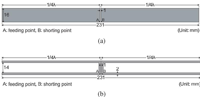
**Figure 1.** (a) Configuration of general two-rectangular patches dipole antenna, (b) back to back symmetric dual-C-shape uniform strips dipole antenna.
