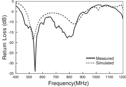
**Figure 7.** Simulated and measured return loss for the proposed.
