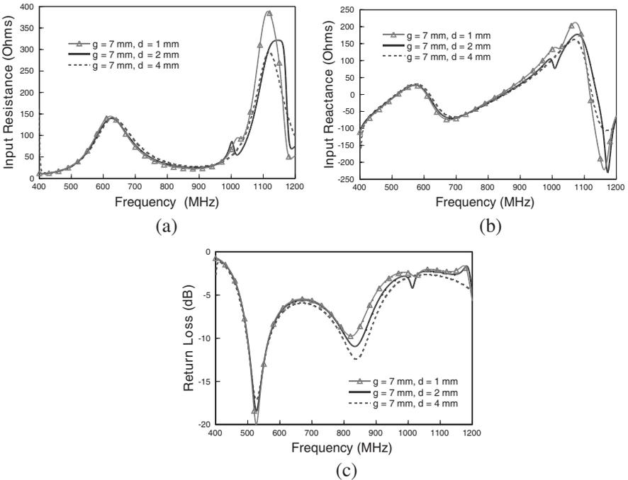
**Figure 5.** Simulated the variation of the proposed antenna with various strips width  $d$  ( $g = 7$  mm). (a) Resistance of the proposed antenna for variation in  $d$ . (b) Reactance of the proposed antenna for variation in  $d$ . (c) Simulated return loss for the proposed antenna with various strips width  $d$  other parameters are the same as Figure 3.
