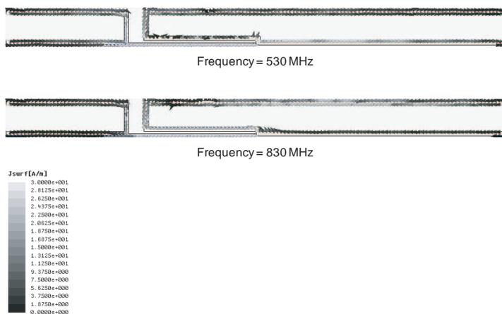
**Figure 6.** Simulated excited surface currents distribution of the resonant mode at (a) 530 MHz, (b) 830 MHz.
