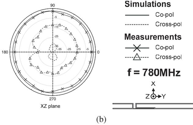
**Figure 8.** Simulated and measured radiation patterns of the proposed antenna in the  $x$ - $y$ ,  $y$ - $z$  and  $x$ - $z$  planes at (a) 540 MHz, (b) 780 MHz.
