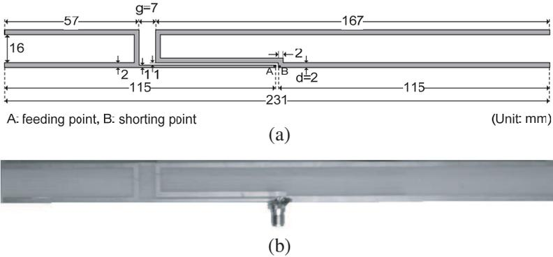
**Figure 3.** (a) Configuration of the printed dipole antenna with back to back asymmetric dual-C-shape uniform strips for DTV applications. (b) Photograph of fabricated antenna with SMA.
