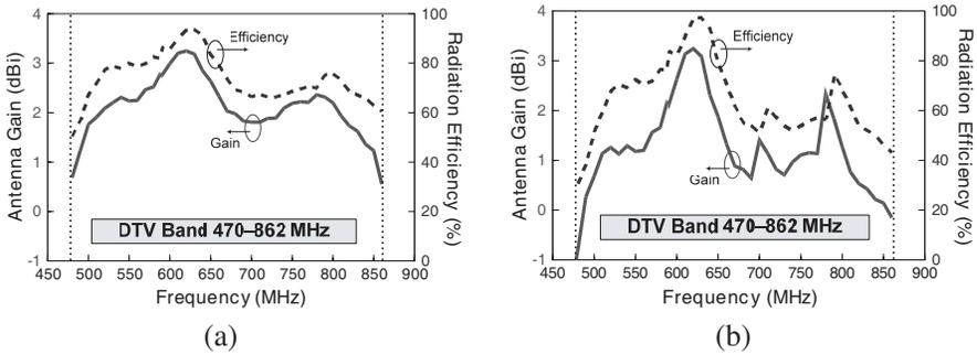
**Figure 9.** Antenna gain and radiation efficiency for the proposed antenna, (a) Simulated. (b) Measured.
