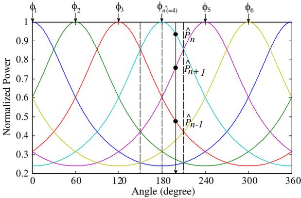
**Figure 2.** Six directive beam patterns.
