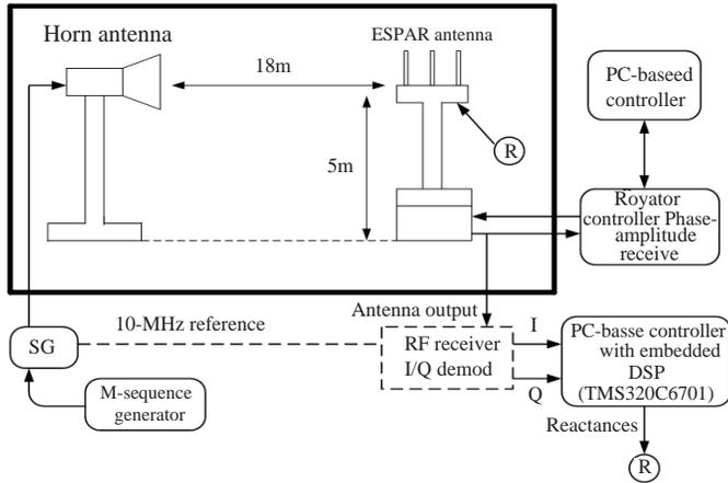
**Figure 10.** Experimental environment and measurement system setup.
