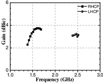
**Figure 8.** Measured antenna gains.
