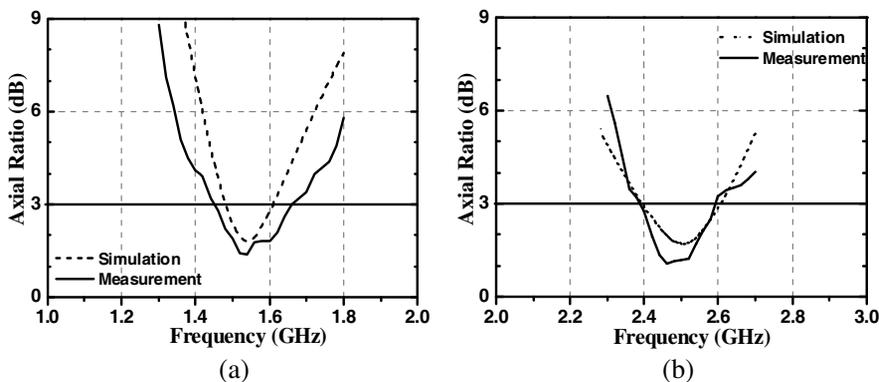
Figure 4. Axial ratio spectrums (a) 1.57 GHz, (b) 2.46 GHz.
