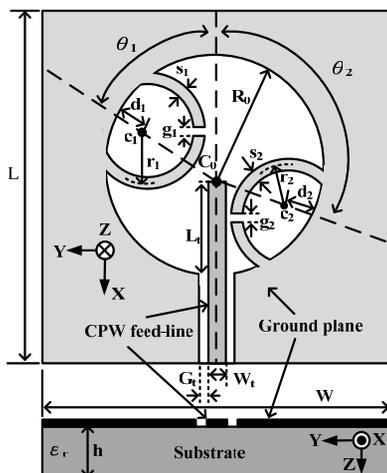
**Figure 1.** Configuration of the proposed CPW-fed slot antenna.
