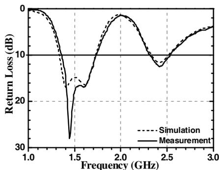
Figure 3. Return loss spectrums of the proposed antenna.
