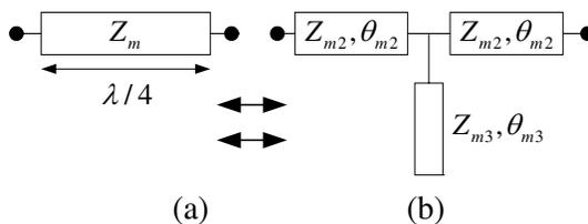
**Figure 3.** (a) Quarter-wave transmission line. (b) Equivalent T-shaped transmission line.
