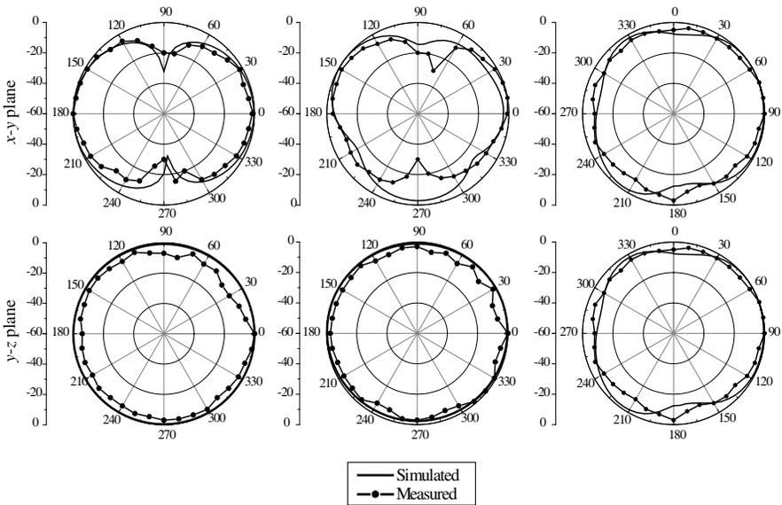
**Figure 10.** The measured and simulated results of antenna radiation pattern.
