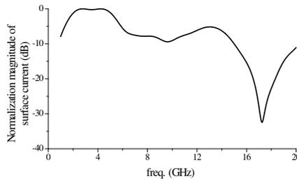
**Figure 2.** The simulated result of current at the end of feeding line.
