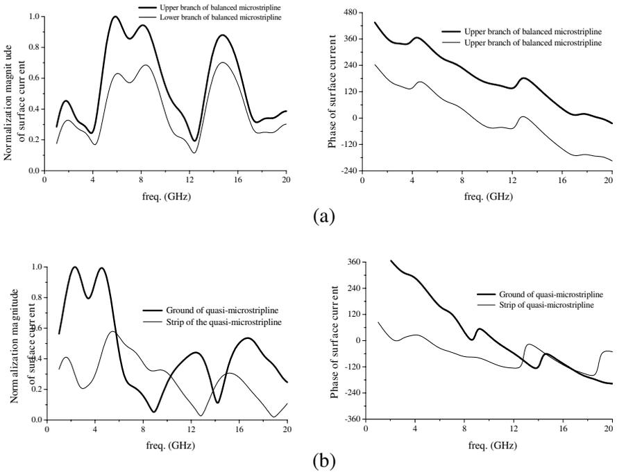
**Figure 7.** The simulated results of surface currents' magnitude and phase for quasi-microstrip-line-to-balanced-microstrip-line. (a) The simulated results of surface currents' magnitude and phase at the end of balanced microstrip-line. (b) The simulated results of surface currents' magnitude and phase at the end of quasi-microstrip-line.
