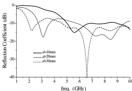
**Figure 4.** The simulated results of reflection coefficient with varying  $d$ .
