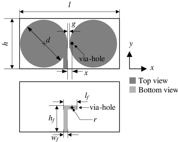
**Figure 1.** Sketch of the proposed antenna with associated geometrical parameters ( $d = 19$  mm,  $w_f = 1.5$  mm,  $h_f = 10.75$  mm,  $l_f = 3.75$  mm,  $r = 2.5$  mm,  $h = 20$  mm,  $l = 40$  mm,  $x = 0.7$  mm,  $g = 0.5$  mm).
