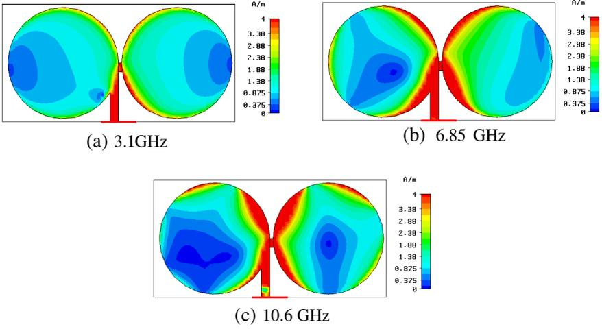
**Figure 3.** The simulated results of surface current on wafers.
