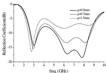
**Figure 5.** The simulated results of reflection coefficient with varying  $g$ .
