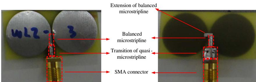
**Figure 6.** The feeding structure of coaxial-line-to-quasi-microstrip-line-to-balanced-microstrip-line.
