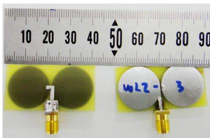
**Figure 8.** The prototype of the proposed antenna.
