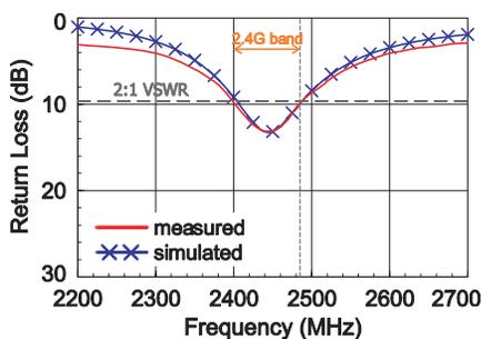
**Figure 3.** Measured and simulated return loss;  $D = 35.5$  mm,  $L = 15$  mm.
