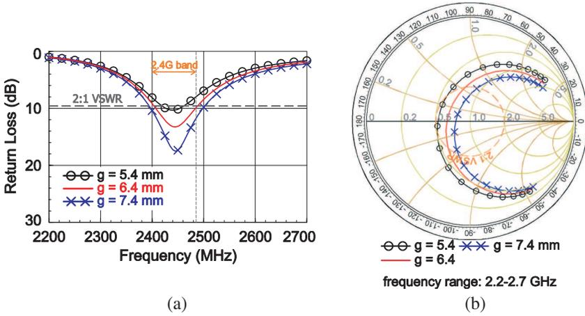
**Figure 5.** Simulated (a) return loss and (b) input impedance on the Smith chart as a function of the distance  $g$  of the air separation.
