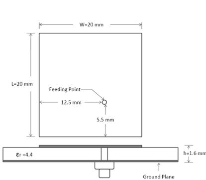
**Figure 1.** Antenna 1 configuration.
