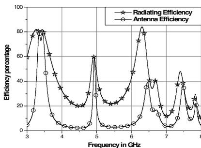
Figure 13. Efficiency versus frequency plot for the antenna 2.
