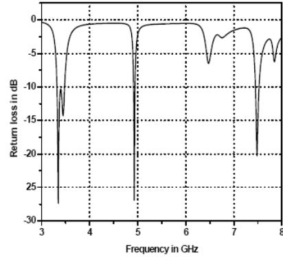
**Figure 4.** Simulated return loss of the antenna 2.
