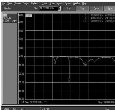
**Figure 16.** Measured return loss of antenna 1.
