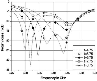
**Figure 7.** Simulated return loss for different values of  $t$ .
