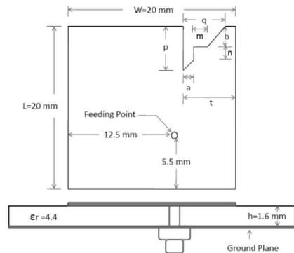
**Figure 2.** Antenna 2 configuration.
