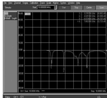
**Figure 17.** Measured return loss of antenna 2.
