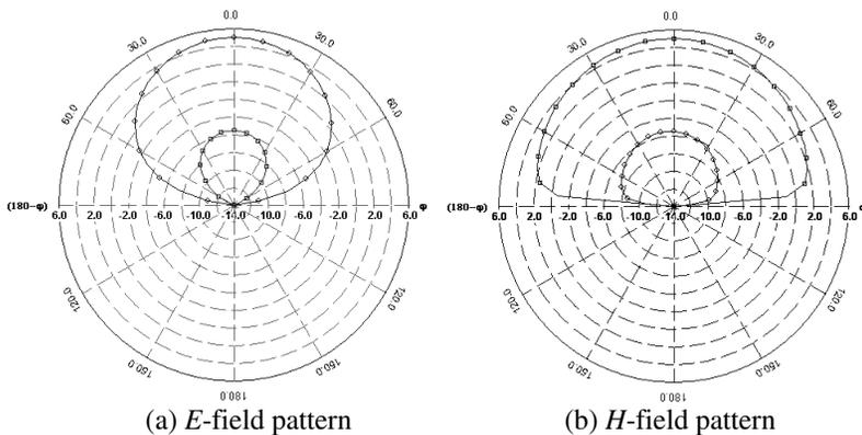
Figure 11. Simulated radiation pattern at 3.45 GHz.
