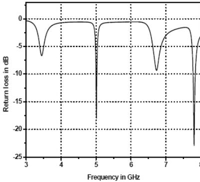
**Figure 3.** Simulated return loss of the antenna 1.
