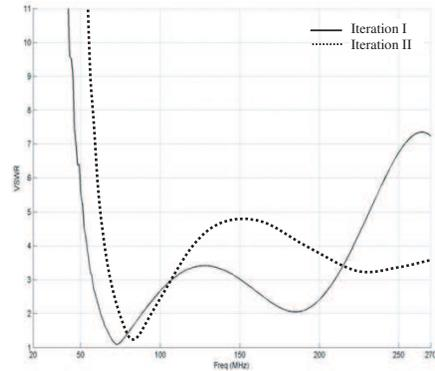
**Figure 5.** Simulated VSWR curves for two iterations.
