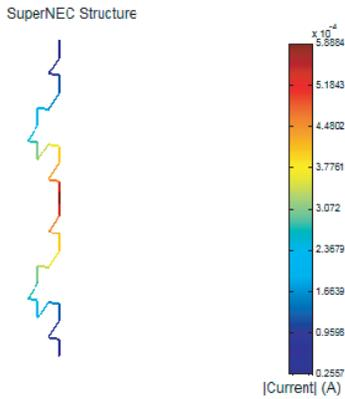
**Figure 4.** Simulated current distribution of the antenna.
