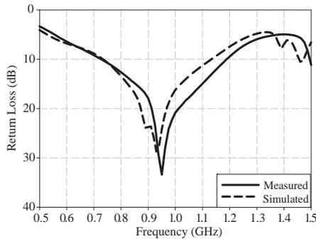
**Figure 9.** Measured and simulated return loss characteristics.
