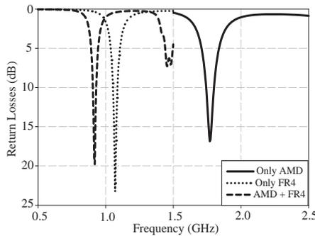
**Figure 5.** Return loss characteristics for three different substrates.
