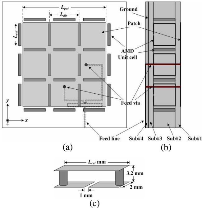
**Figure 1.** The proposed antenna structure in (a) top view, (b) side view, and (c) a unit cell.
