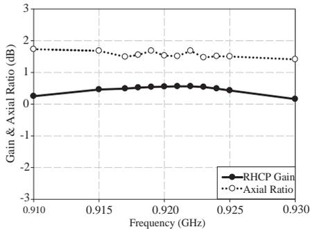
**Figure 11.** Measured peak gain and axial ratio.
