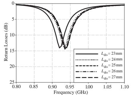
**Figure 7.** Return loss characteristics for the various distances between unit cells  $L_{\text{dis}}$ .
