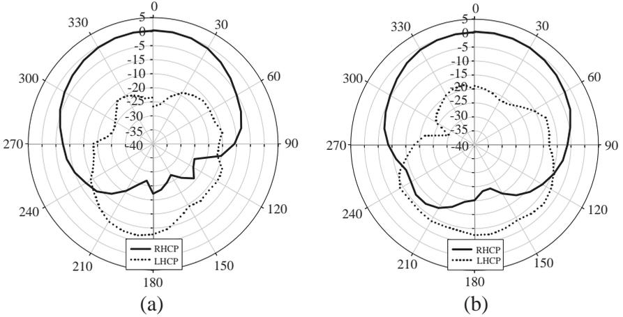
**Figure 10.** Measured radiation patterns (a)  $x$ - $z$  plane and (b)  $y$ - $z$  plane.
