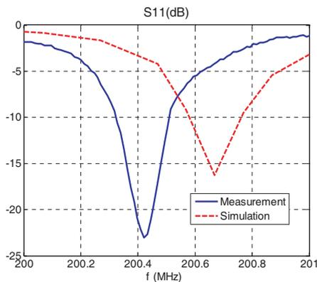
Figure 8. Measured and computed return loss (dB).
