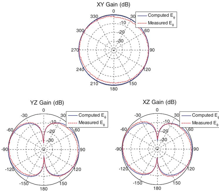
**Figure 9.** Measured and computed radiation patterns at the resonant frequency.
