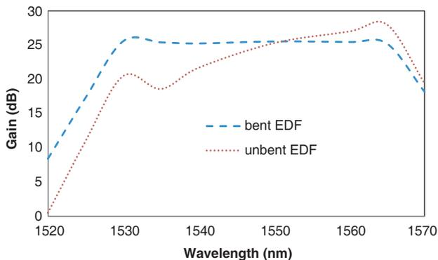
**Figure 5.** Gain spectrum of the EDFA with and without macro-bending at EDF length of 2.5 m.
