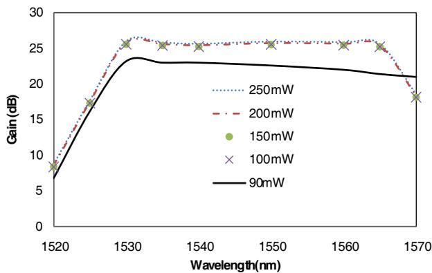
**Figure 7.** Gain spectrum of the proposed EDFA at different pump powers.
