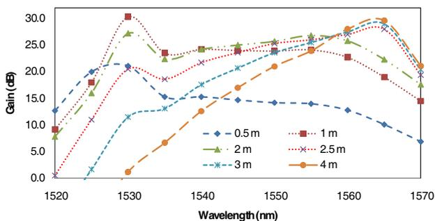
**Figure 3.** Gain spectrum at different EDF lengths (without macro bending).
