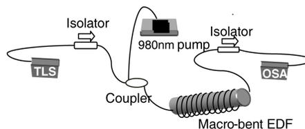
**Figure 1.** Configuration of the proposed gain-flattened C-band EDFA.
