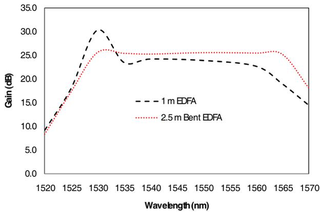
**Figure 6.** Comparison of gain spectrum of the proposed gain flattened EDFA with standard C-band EDFA.
