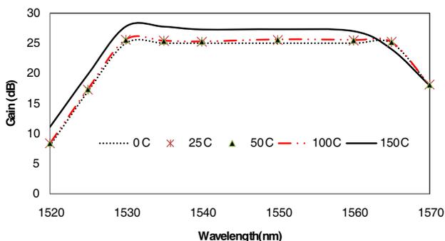
**Figure 10.** Gain profile of 2.5 m macro-bent EDFA at different temperatures.
