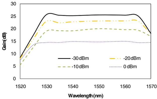
**Figure 8.** Gain spectrum of 2.5 m bent EDF at various input signal powers.
