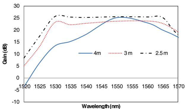
**Figure 4.** Gain spectrum at different EDF lengths (with macro bending).
