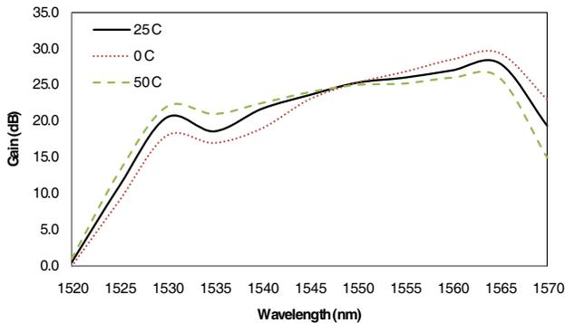
**Figure 9.** Gain profile of 2.5 m un-bent EDFA at different temperatures.
