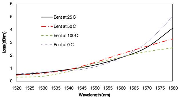
**Figure 2.** Loss spectrum of the bent EDF with 6.5 mm bending radius at different temperatures.
