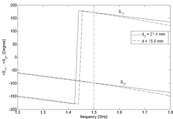
**Figure 8.** Comparing the angle of  $S$  parameters of designed NCTL No. 2 (O.C. 2-Port,  $d = 15$  mm) with those of corresponding UCTL.
