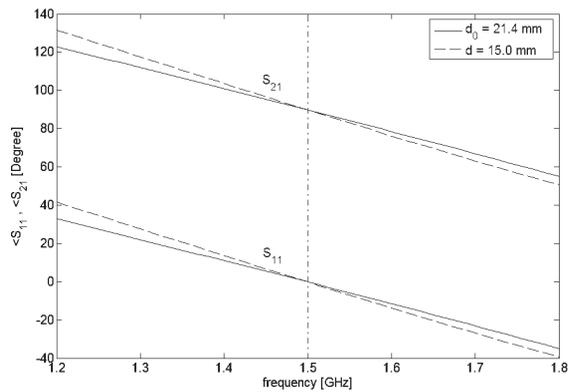
**Figure 10.** Comparing the angle of  $S$  parameters of designed NCTL No. 3 (S.C. 2-Port,  $d = 15$  mm) with those of corresponding UCTL.
