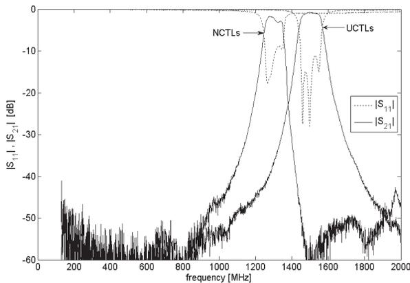
**Figure 12.** The measured  $S$  parameters of two conventional and compacted edge-coupled BPFs.
