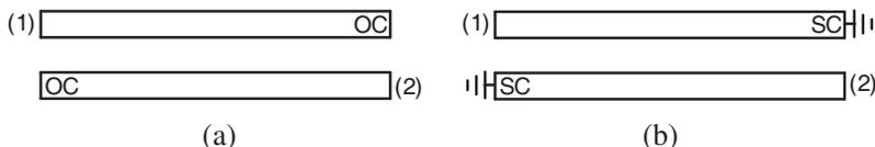
**Figure 3.** Longitudinal view of two special cases of coupled transmission lines (a) open circuited, (b) short circuited.
