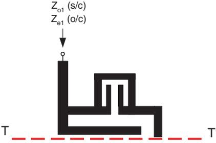
**Figure 2.** Bisected proposed coupled transmission-line.
