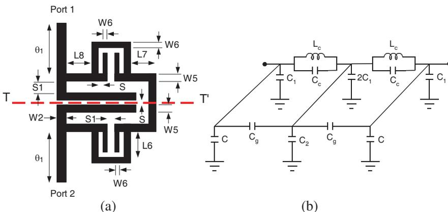
**Figure 1.** (a) The proposed coupled microstrip transmission-line model using fractal technique; (b) its equivalent circuit model.
