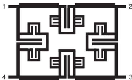
**Figure 4.** Schematic diagram of the proposed branch-line coupler.
