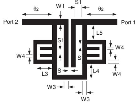
**Figure 3.** The horizontal coupled transmission-line in the branch-line coupler.
