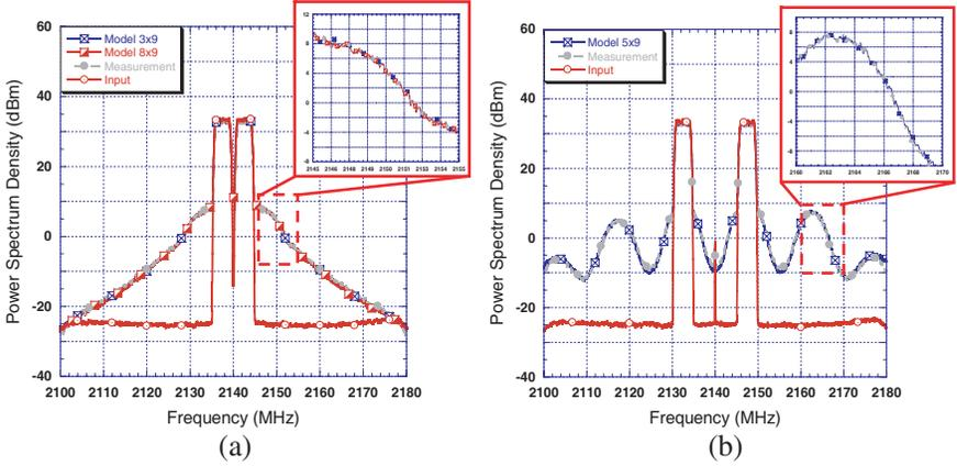
**Figure 9.** Model's performance assessment in frequency domain (a) WCDMA 11 signal using model parameters  $3 \times 9$  (successive sweep),  $8 \times 9$  (simultaneous sweep) along with the measured spectrum. (b) WCDMA 1001 signal using model parameters  $5 \times 9$  (simultaneous and successive sweeps) along with the measured spectrum.
