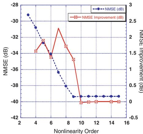
**Figure 5.** Calculated NMSE and NMSE improvement as a function of the model's nonlinearity order under memory effects free behavior.
