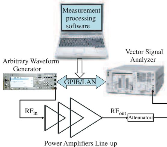
**Figure 1.** Experimental setup for DUT characterization.
