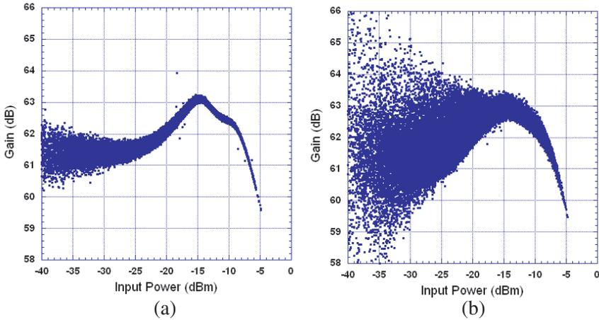
**Figure 3.** Measured AM/AM characteristics of the DUT. (a) under WCDMA 1-Carrier drive. (b) under WCDMA 4-Carrier (1001) drive.
