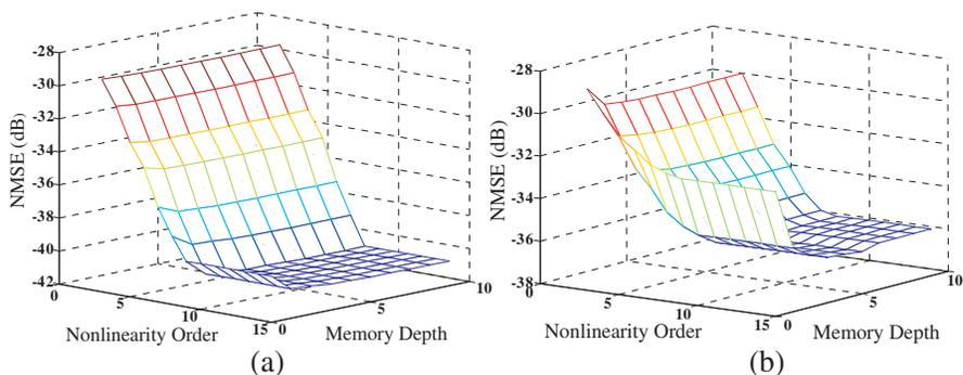
**Figure 8.** Calculated NMSE for the DUT model versus the nonlinearity order and the memory depth. (a) WCDMA11 signal. (b) WCDMA 1001 signal.
