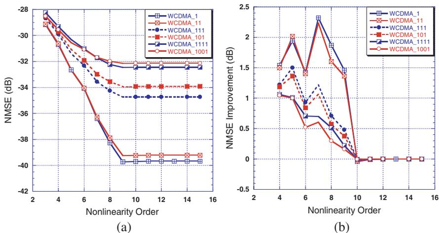
**Figure 6.** Calculated performance of the models versus the nonlinearity order under the actual drive signal. (a) NMSE. (b) NMSE improvement.
