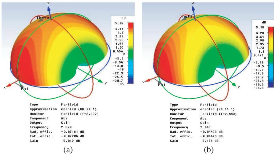
**Figure 12.** Radiation patterns (3D Views) of FRC-1 DRAs with  $\epsilon_r = 20$ . (a) Conventional FRC DRA. (b) Modified FRC-1 DRA.
