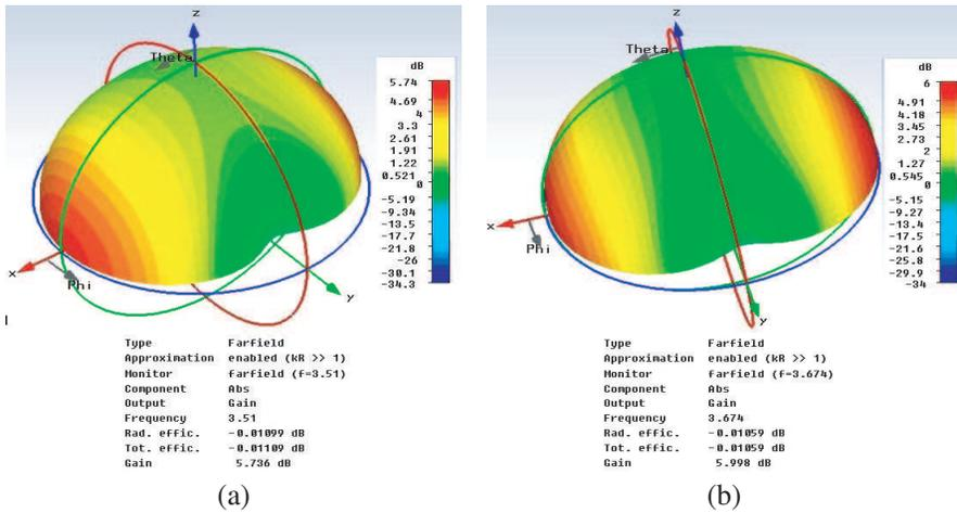
**Figure 11.** Radiation patterns (3D Views) of FRC-1 DRAs with  $\epsilon_r = 8$ . (a) Conventional FRC DRA. (b) Modified FRC-1 DRA.
