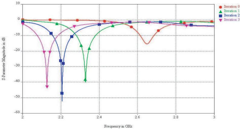
**Figure 4.** Variation in return loss with frequency for conventional FRC DRAs.
