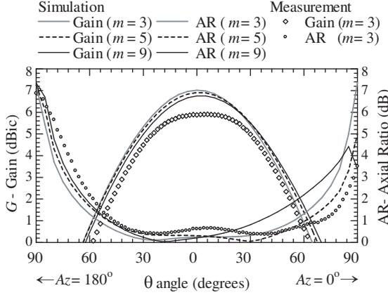
**Figure 8.** Simulated and measured gain and AR vs. theta angle (radiation pattern) in the theta plane ( $Az = 0^\circ$  and  $180^\circ$ ) ( $x$ - $z$  plane) at  $f = 1.285$  GHz.
