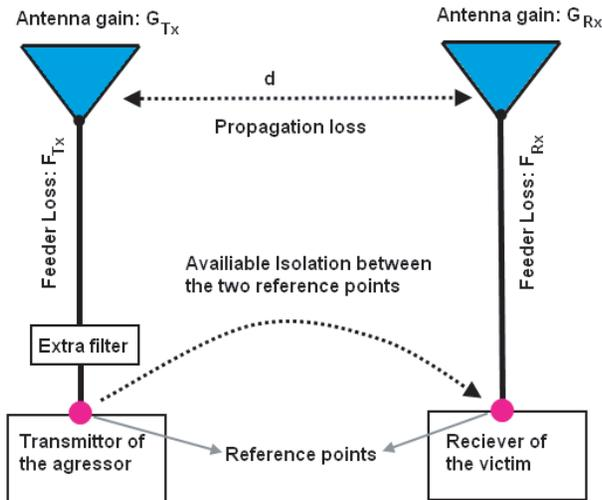
**Figure 1.** Isolation requirement between transmitter and receiver.
