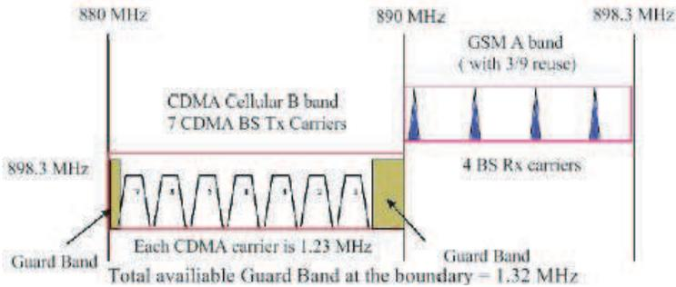
**Figure 3.** Frequency allocation for CDMA and GSM systems.
