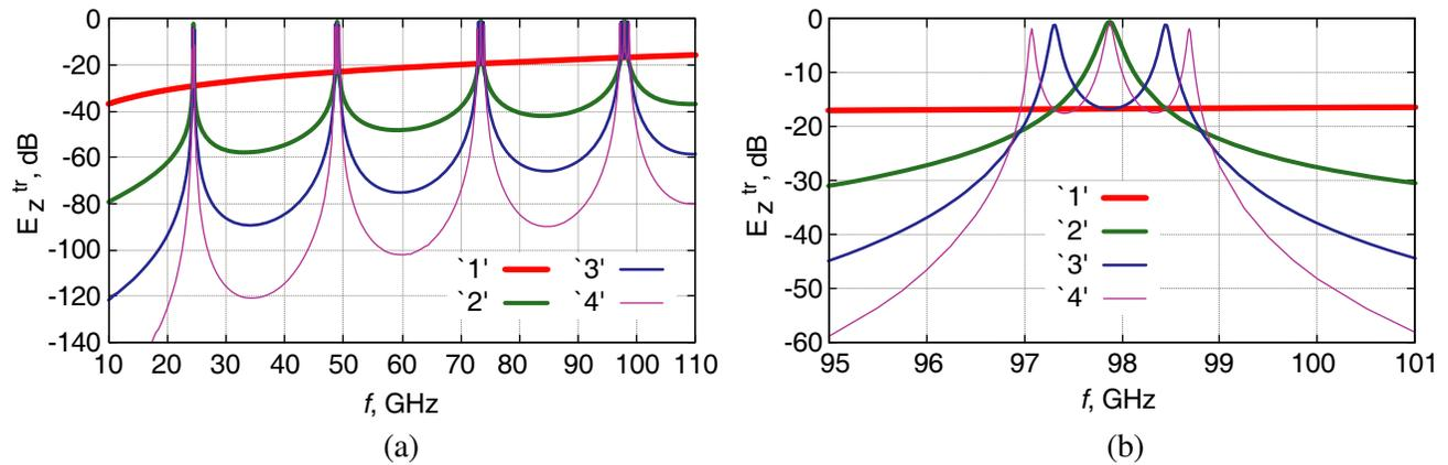
**Figure 3.** Full-wave simulated transmission spectra of  $E_z^{tr}$  field component (a) in the band of  $f = 10 - 110$  GHz and (b) at the 4th-order resonant transmission peak ( $p_4$ ) for the assemblies  $G_n$  of  $n = 1, 2, 3, 4$  gratings presented in Figure 1 with interlayer spacings  $b = 6.00$  mm (rejected polarization, curves ‘1’ to ‘4’, respectively).
