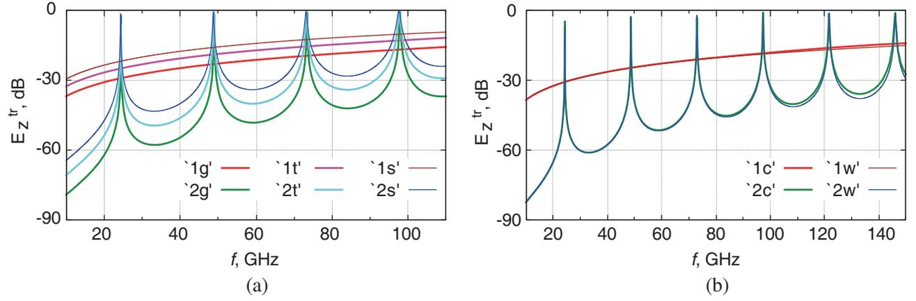
**Figure 5.** (a) FlexPDE vs asymptotic solutions for  $G_n$  ( $n = 1, 2$ ) multilayer gratings of (a) strips of width  $w = 0.17$  mm and thickness  $t = 0.10$  mm and  $0.04$  mm (FlexPDE, curves with suffix ‘g’ and ‘t’, respectively), and  $t = 0$  mm (‘gs’ solutions, curves with suffix ‘s’), and (b) wires of the diameter  $w = 0.17$  mm (FlexPDE and ‘gw’ solutions, curves with suffix ‘c’ and ‘w’, respectively).
