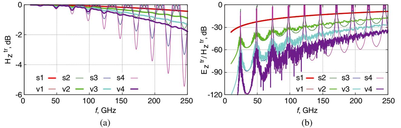
**Figure 9.** (a) Transmission spectra of the waves of  $H_z$  polarization and (b) polarization extinction ratio  $E_z/H_z$  computed for strip-grating assemblies  $G_n$  of  $n = 1$  to 4 layers in the model with roughness of gratings specified by parameters  $\sigma = 0.3$  mm and  $K = 900$  as compared to the ideal case of gratings at  $\sigma = 0$  (‘s’ model, curves ‘v1’ to ‘v4’ vs ‘s1’ to ‘s4’, respectively).
