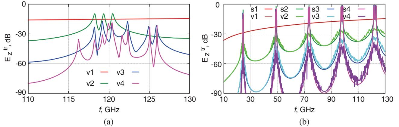
**Figure 8.** Transmission spectra of the waves of  $E_z$  polarization computed for strip-grating assemblies  $G_n$  of  $n = 1$  to 4 layers with roughness of gratings specified by Gaussian distribution with standard deviation  $\sigma = 0.15$  mm using the random sampling of (a)  $K = 3$  and (b)  $K = 900$  “pixel patches” as compared to the ideal case of  $\sigma = 0$  (‘s’ model, curves ‘v1’ to ‘v4’ vs ‘s1’ to ‘s4’, respectively).
