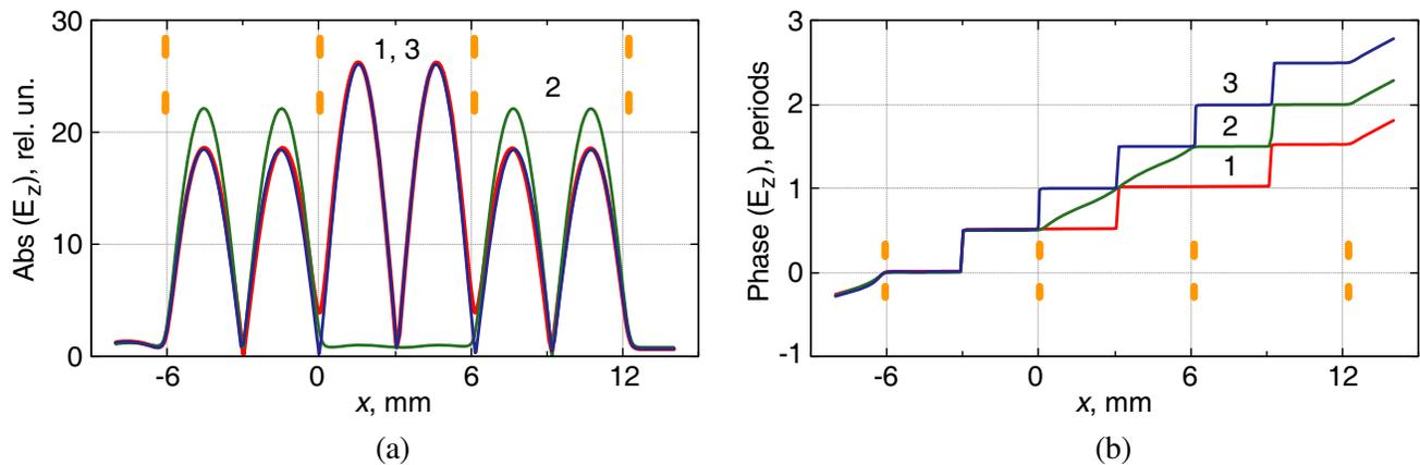
**Figure 4.** (a) Amplitude and (b) phase of  $E_z$  field component of plane wave propagating through a 4-layer grating structure  $G_4$  (dash lines show locations of gratings) at the resonant frequencies  $f_{p_2}^{(k)}$  of triple-split 2nd-order transmission peak  $p_2$  (see curve ‘4’ in Figure 3) where  $f_{p_2}^{(k)} = 48.563, 48.953,$  and  $49.351$  GHz ( $k = 1, 2, 3$ , curves 1 to 3, respectively).
