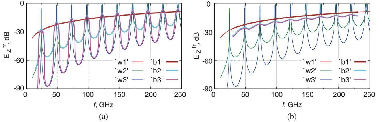
**Figure 7.** Transmission spectra  $E_z^{tr}$  computed for the wire-grid assemblies  $G_n$  ( $n = 1, 2, 3$ ) if measured with monochromatic (curves ‘w1’ to ‘w3’) and broadband detector (curves ‘b1’ to ‘b3’, respectively) at the detector bandwidth (a)  $\delta f = 5$  GHz and (b)  $\delta f = 20$  GHz.
