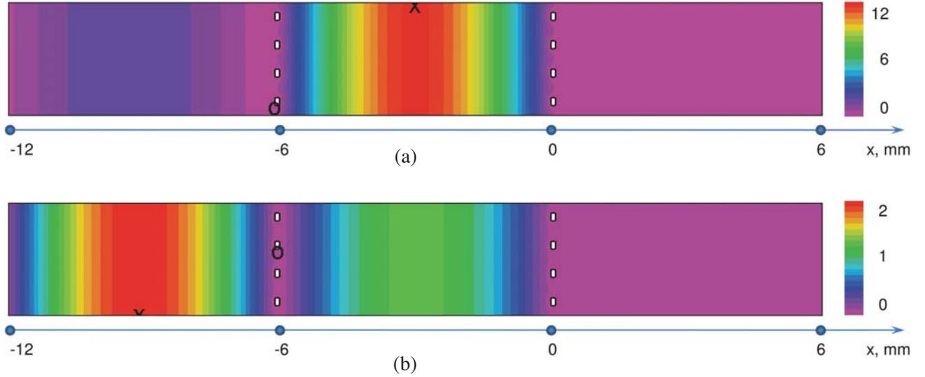
**Figure 2.** The amplitude of simulated  $E_z(x, y)$  field component in a two-layer grid structure  $G_2$  with interlayer spacing  $b = 6.00$  mm at the frequency (a)  $f = 24.5$  GHz and (b)  $f = 24.7$  GHz (the case of rejected polarization near the first resonant transmission peak frequency  $f_{p1} = 24.4787$  GHz, symbols “o” and “x” on the plot show the locations of minima and maxima).
