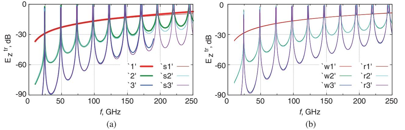
**Figure 6.** (a) Full-wave FlexPDE vs ‘s’ model asymptotic solutions for strip grating  $G_n$  structures (curves ‘1’ to ‘3’ vs ‘s1’ to ‘s3’,  $n = 1, 2, 3$ , respectively) and (b) ‘w’ model asymptotic solutions vs regularization-based ‘r’ model results (curves ‘w1’ to ‘w3’ vs ‘r1’ to ‘r3’, respectively).
