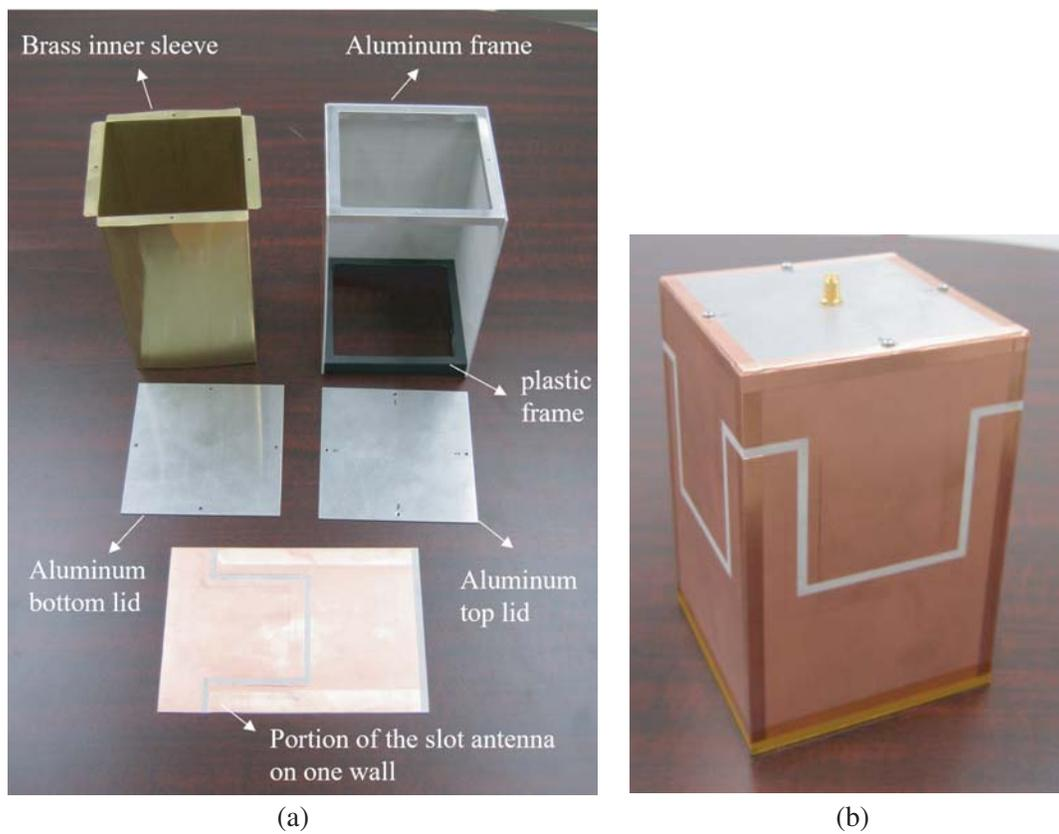
**Figure 4.** The antenna assembly. (a) Major arts. (b) Finished prototype.
