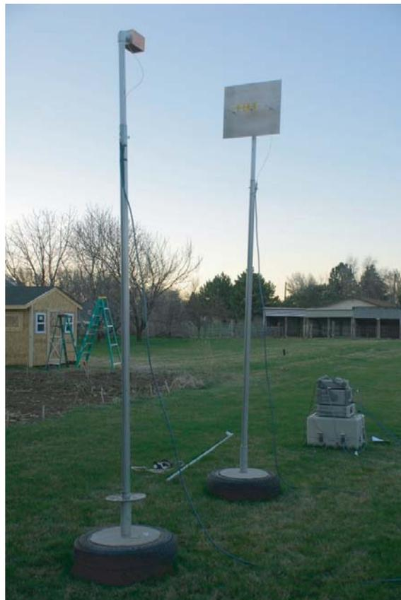
**Figure 10.** Field setup for range test of 1.5U CubeSat antenna.
