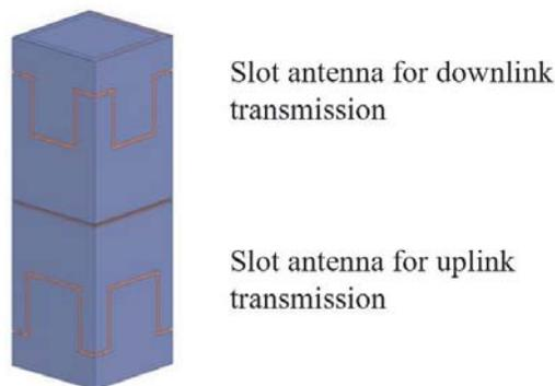
**Figure 3.** Proposed design of circularly polarized slot antenna for 3U CubeSat.
