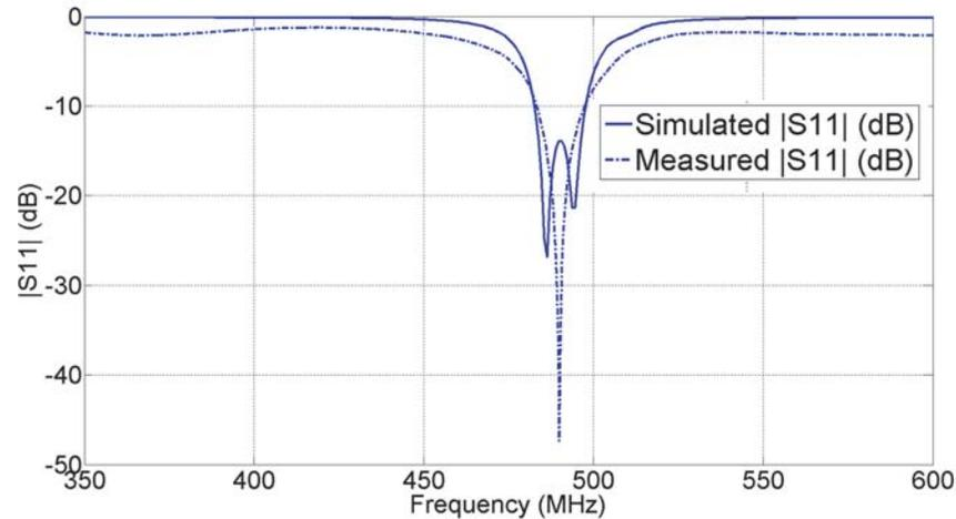
**Figure 9.** Simulated and measured reflection coefficient for lower slot (uplink).
