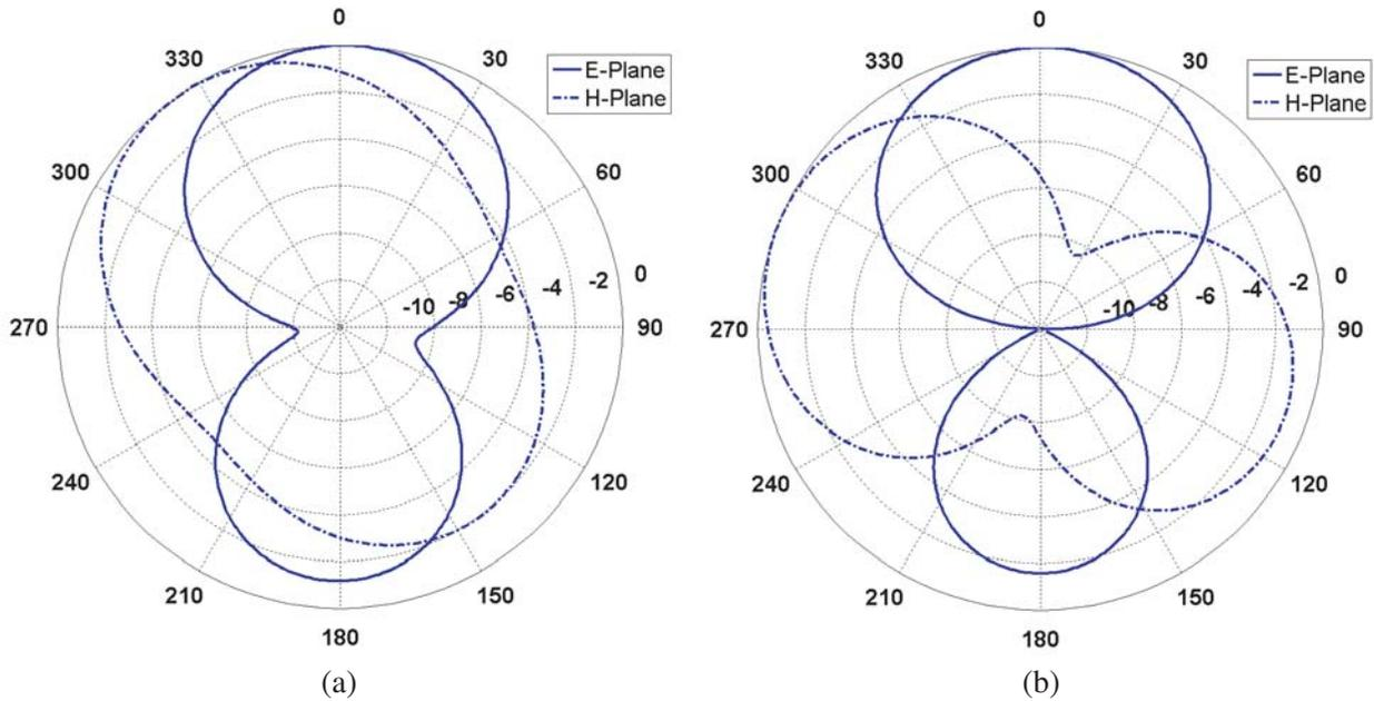
Figure 7. Radiation patterns. (a) Uplink. (b) Downlink.
