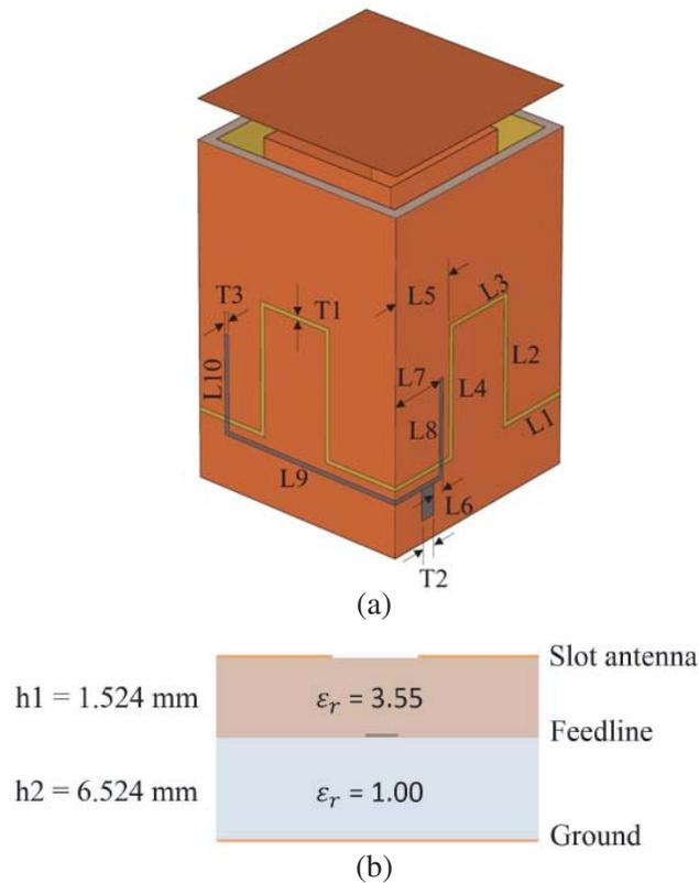
**Figure 2.** Details of the antenna geometry and layer information. (a) Antenna and feedline. (b) Layer information.
