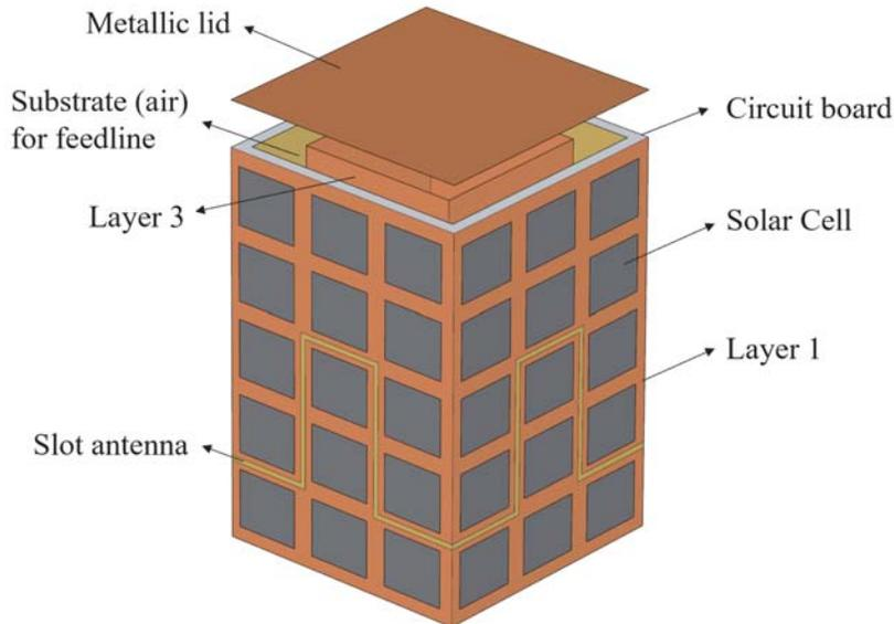
**Figure 1.** A UHF slot antenna on the solar panel of 1.5U CubeSat.
