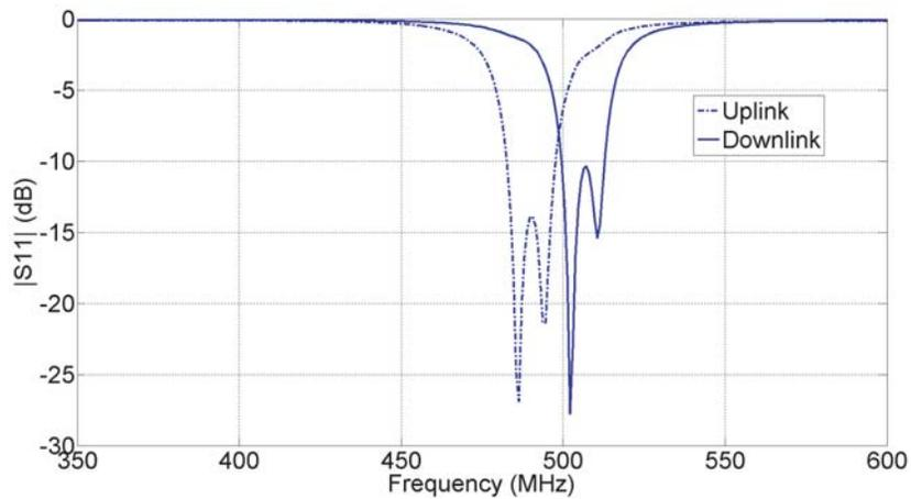
**Figure 6.** Reflection coefficient for uplink and downlink channel slots.
