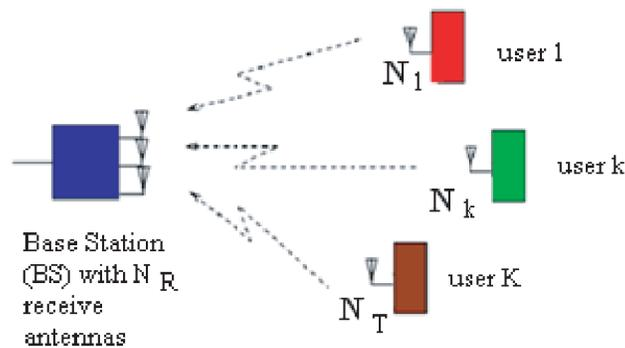
**Figure 2.** Multi-user massive MIMO.
