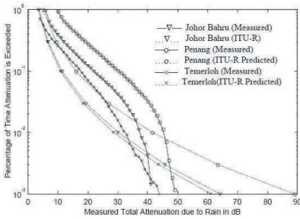
**Figure 5.** Rain attenuation distribution measured at 15 GHz frequency over microwave links at Johor Bahru, Penang and Temerloh and those predicted by ITU-R.
