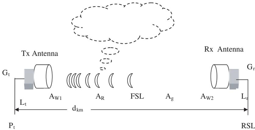
**Figure 1.** Link budget for a terrestrial line-of-sight radio link.
