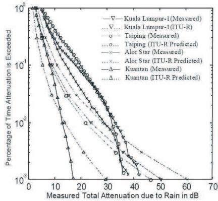
**Figure 6.** Rain attenuation distribution measured at 15 GHz frequency over microwave links at Kuala Lumpur -1, Taiping, Alor star and Kuantan and those predicted by ITU-R.
